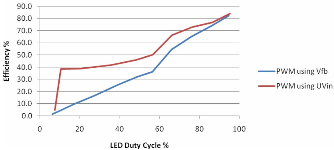
1kHz Strobe - Converter Efficiency
