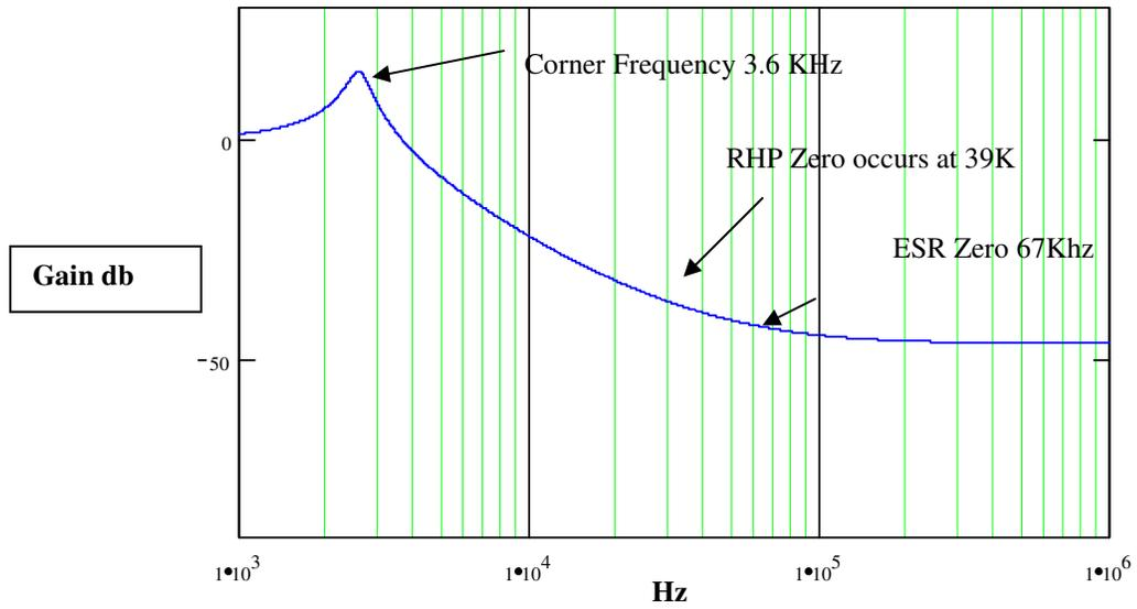
**Diagram 2 Gain of a boost filter**
