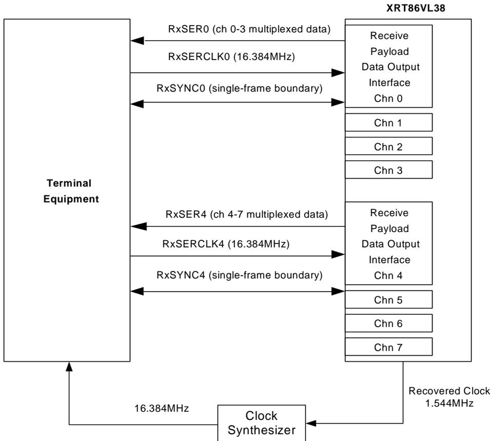
Terminal Equipment will need to supply a 16.384MHz high-speed clock to the RxSERCLK pin on Channel 0 and Channel 4 as the timing reference for the backplane interface. If the receive slip buffer is enabled, Terminal Equipment should also supply a single-frame boundary pulse on the RxSYNC pin for the framer to output the beginning of a multiplexed frame.
