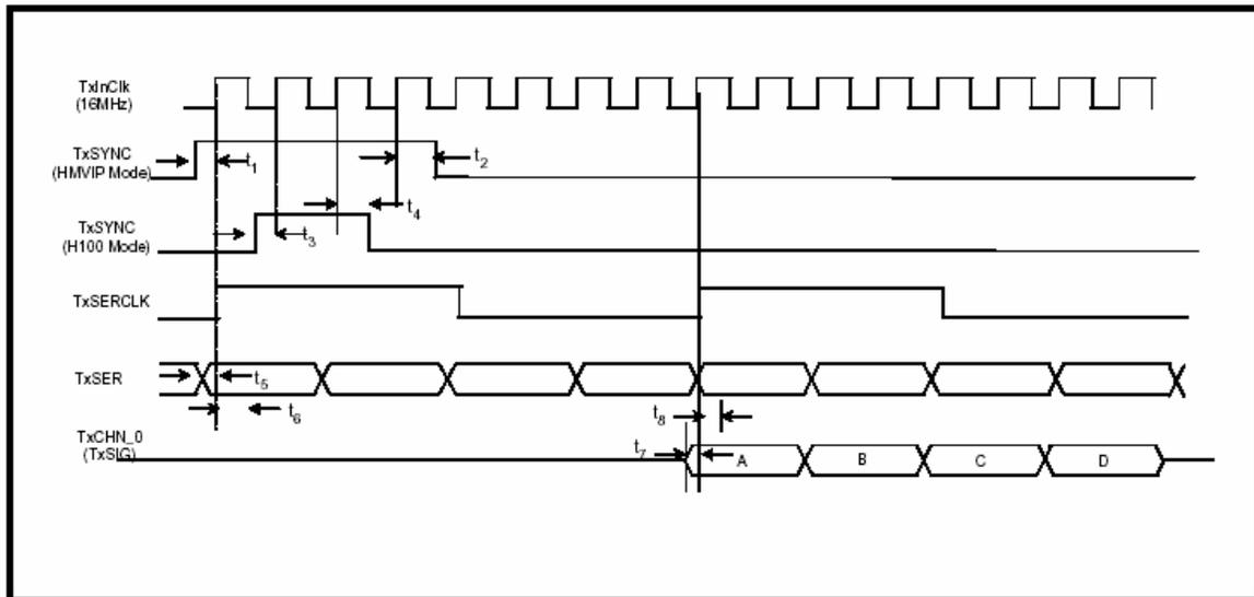
**NOTE:** Setup and Hold time is not valid from TxInClk to TxSERCLK as TxInClk is used as the timing source for the back plane interface and TxSERCLK is used as the timing source on the line side.
