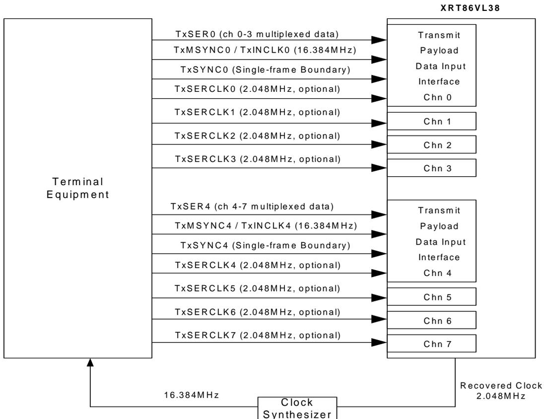
Terminal Equipment will need to supply a 16.384MHz clock to the TxMSYNC/TxINCLK pin on Channel 0 and Channel 4 as the high-speed bus input clock. (In high-speed mode, TxMSYNC is referred to as the TxINCLK signal from here on). In addition, Terminal Equipment should supply a single-frame boundary pulse on the TxSYNC pin for the framer to locate the beginning of the multiplexed frame.
