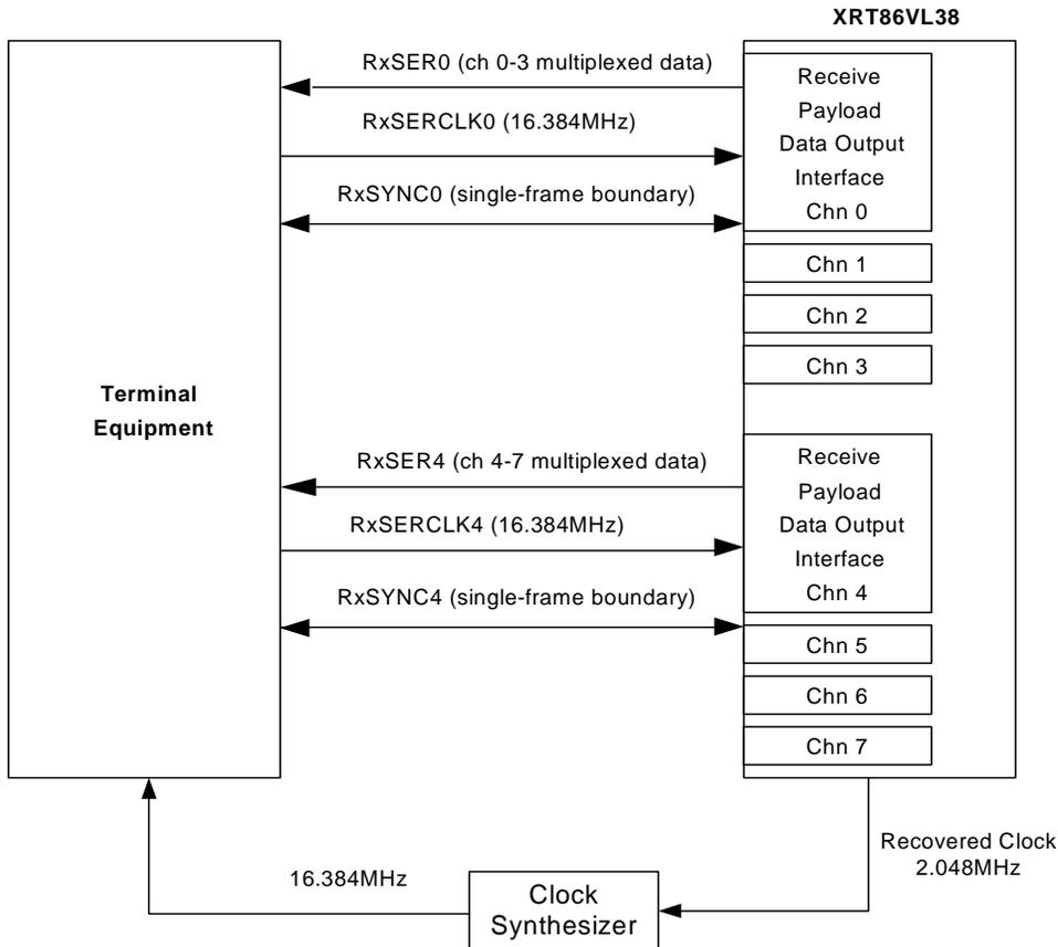
Terminal Equipment will need to supply a 16.384MHz high-speed clock to the RxSERCLK pin on Channel 0 and Channel 4 as the timing reference for the backplane interface. If the receive slip buffer is enabled, Terminal Equipment should also supply a single-frame
