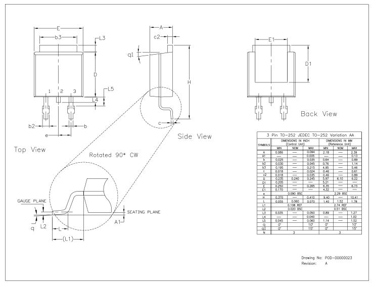
Figure 5: SPX2945 Mechanical Dimensions–3-Pin TO-252
