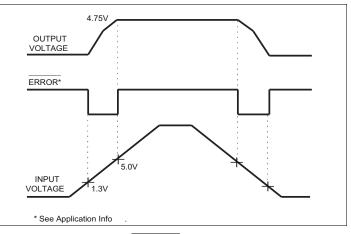
Figure 4: ERROR Output Timing
