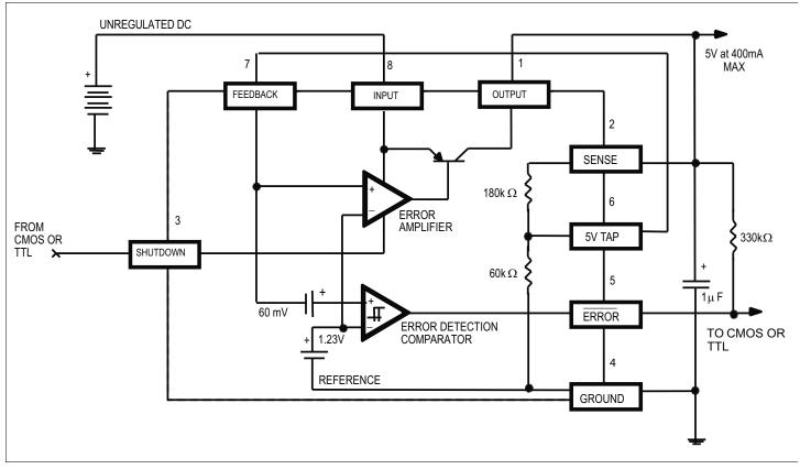
Figure 3: SPX2945 Block Diagram
