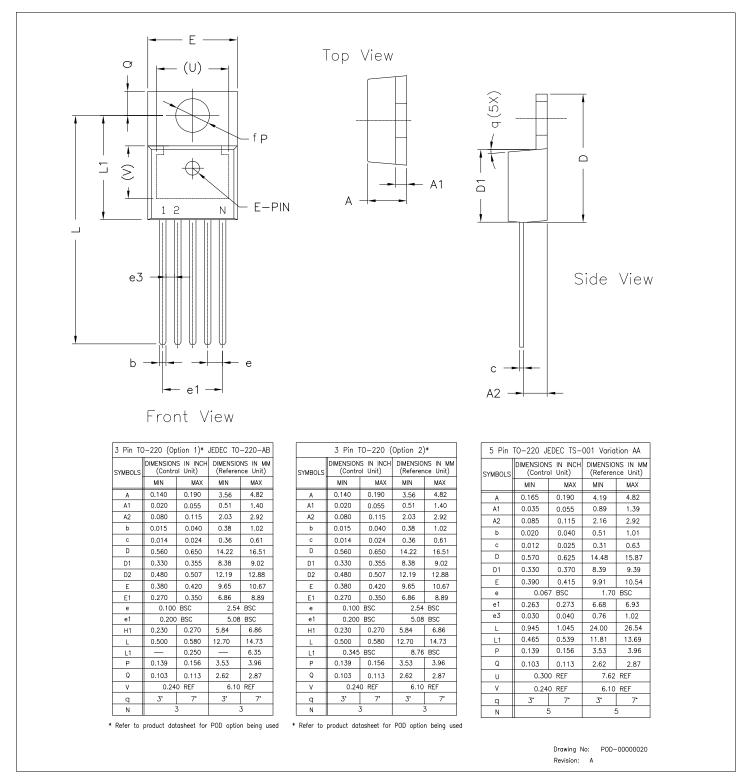
Figure 6: SPX2945 Mechanical Dimensions–5-Pin TO-220
