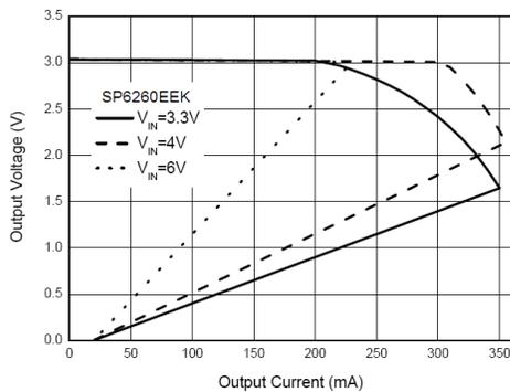
Fig. 8: Output Voltage vs. Output Current SP6260EEK (3.0V)
