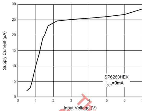
Fig. 15: Supply Current vs. Input Voltage SP6260HEK (1.2V)
