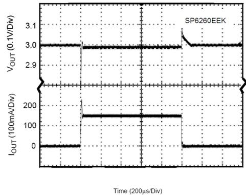
Fig. 22: Line Transient SP6260EEK (3.0V)
