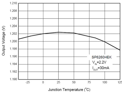
Fig. 13: Output Voltage vs. Junction Temperature SP6260HEK-L (1.2V)
