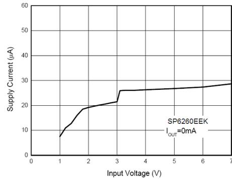
Fig. 16: Supply Current vs. Input Voltage SP6260EEK (3.0V)
