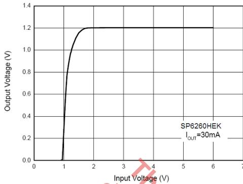
Fig. 9: Output Voltage vs. Input Voltage SP6260HEK (1.2V)
