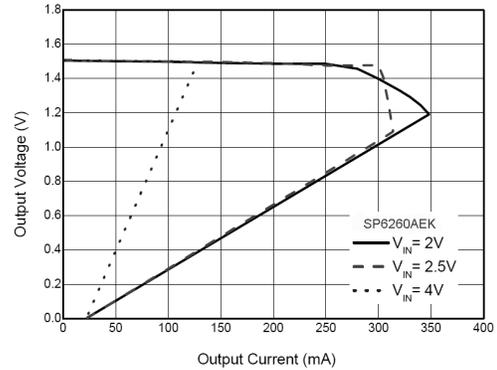
Fig. 5: Output Voltage vs. Output Current SP6260AEK (1.5V)
