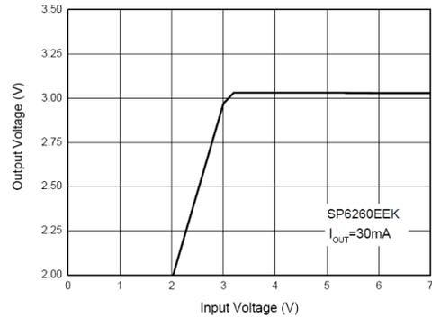
Fig. 10: Output Voltage vs. Input Voltage SP6260EEK (3.0V)
