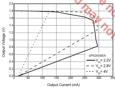
Fig. 6: Output Voltage vs. Output Current SP6260BEK (1.8V)
