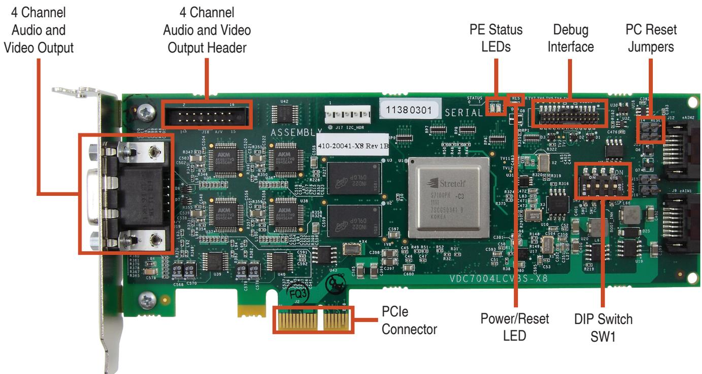
The VDC7004 is available as a production-ready OEM unit for volume production and can be ordered in either full height or low profile bracket configurations.
