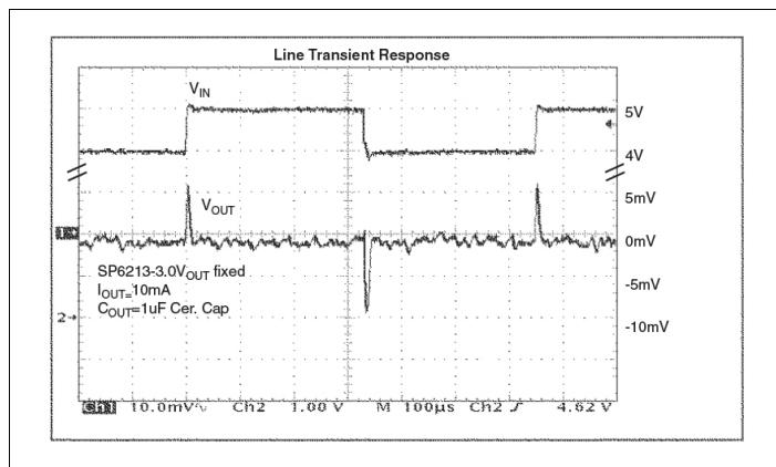
Figure 33: Line Transient Response ( $V_{IN} = 4V$ ,  $I_{OUT} = 10mA$ )
