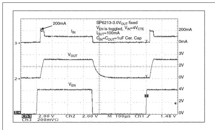
Figure 27: Inrush Current (V<sub>IN</sub> = 4V, I<sub>OUT</sub> = 100mA)
