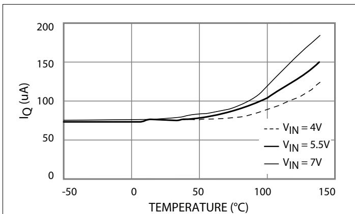
Figure 9: Quiescent Current vs Temperature ( $I_{\text{OUT}} = 0\text{A}$ )
