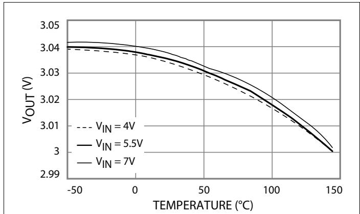
Figure 6: Output Voltage vs Temperature ( $I_{\text{OUT}} = 10\text{mA}$ )
