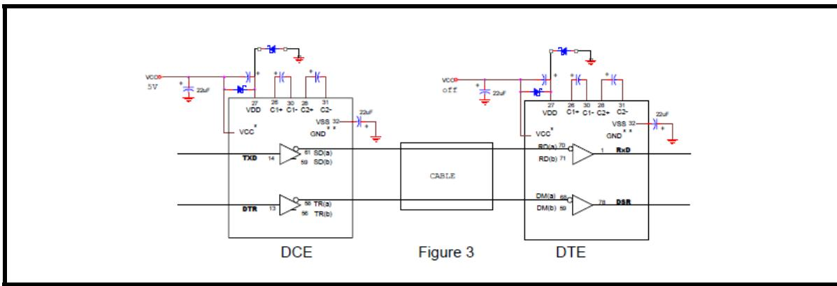
The anode of the Schottky is tied to ground and the cathode to Vdd
