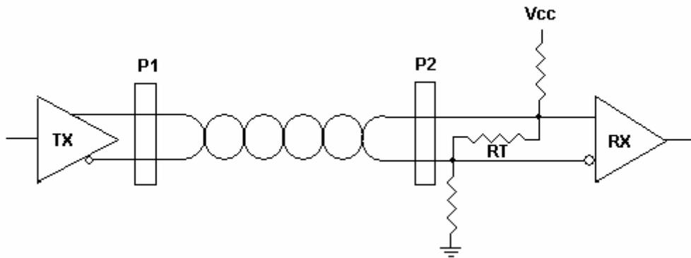
**Figure 2. Receiver Termination and Biasing network configuration**
