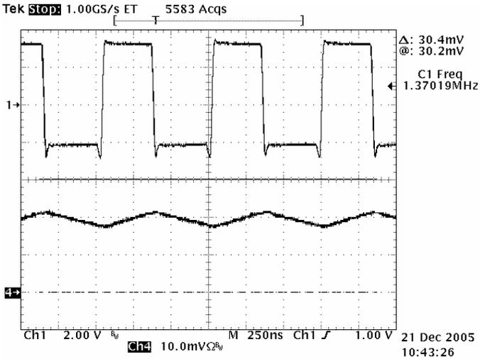
**Channel 1 Switch node Channel 2 is Inductor Current I<sub>L</sub>
