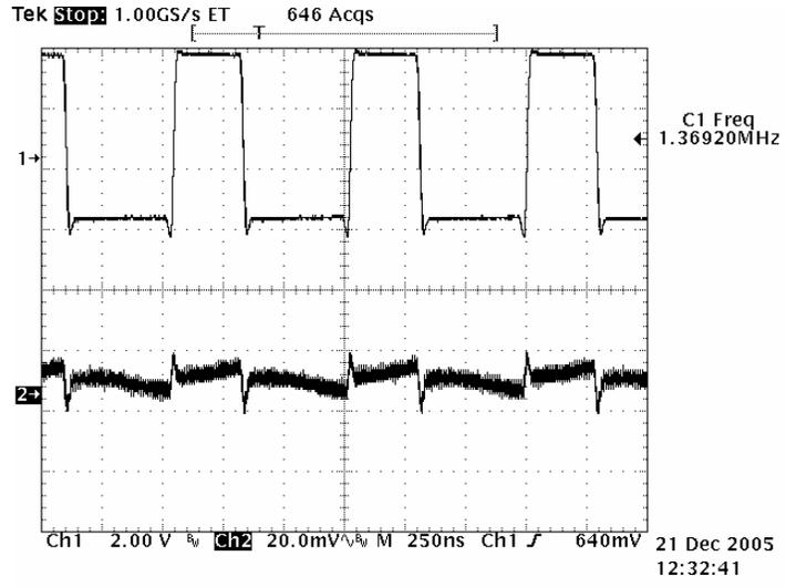
Channel 2  $V_{out}$  ripple Channel 1 Switch Node
