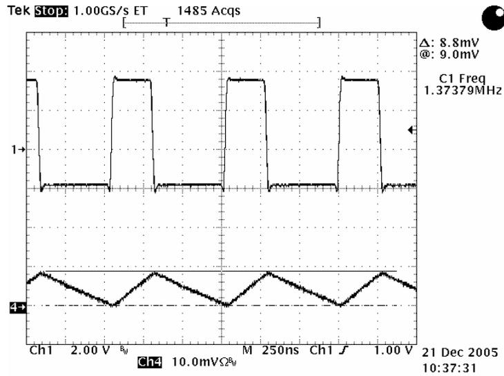
**Channel 1 Switch node Channel 2 is Inductor Current  $I_L$
