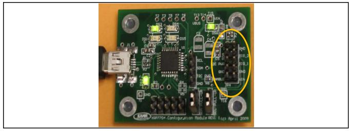
Figure 2: XRP77XXEVB-XCM JP4 Pin Assignment
