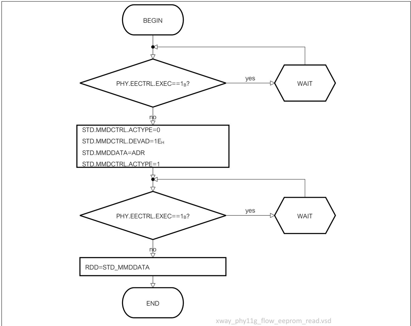
Figure 21 Flow-Chart for an Indirect EEPROM Read Cycle Via MDIO-MMD Access
