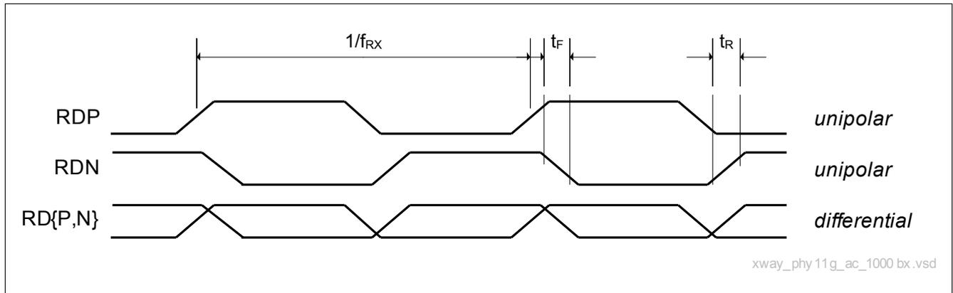
Figure 52 Receive Timing Diagram of the 1000BASE-X
