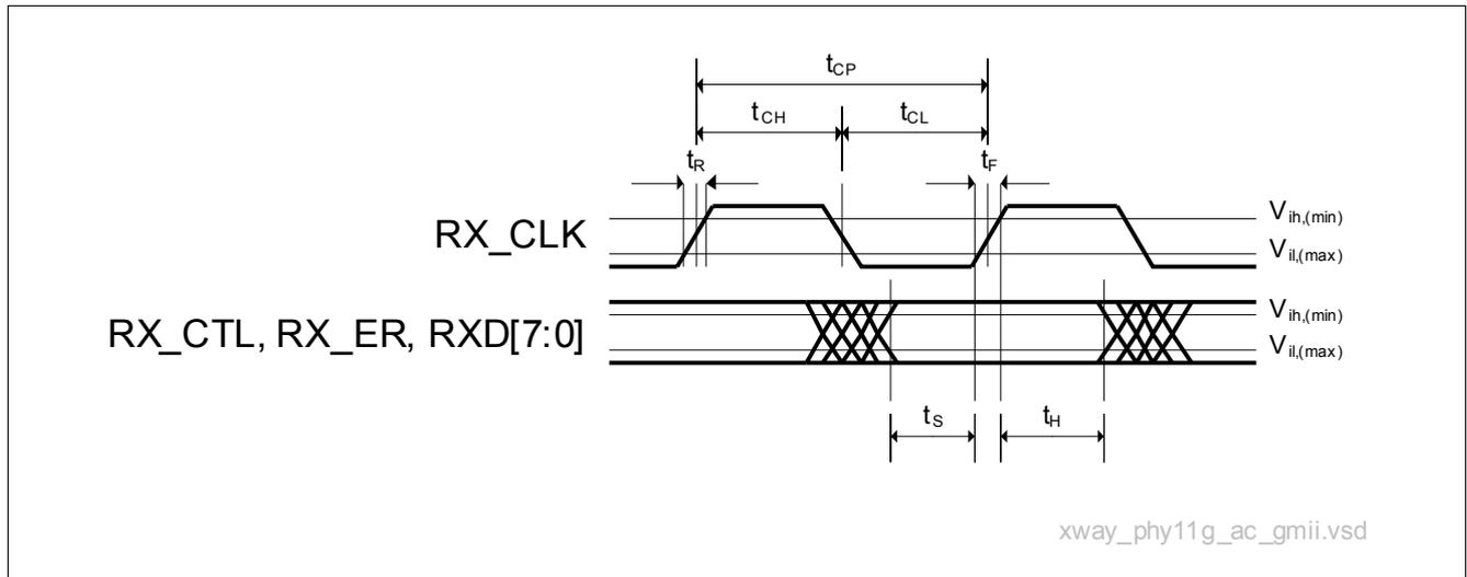
Figure 46 Receive Timing Diagram of the GMII
