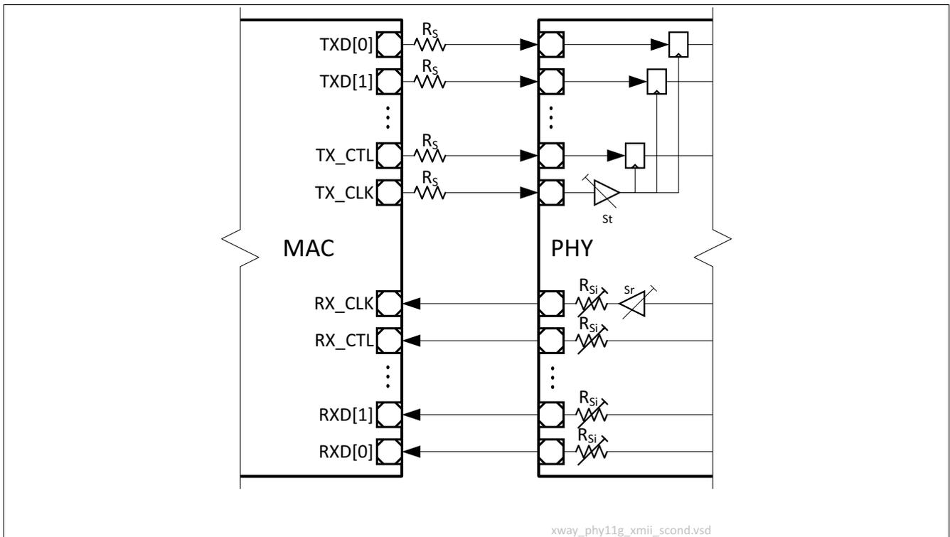
Figure 10 xMII Signal Conditioning between MAC and GPY112
