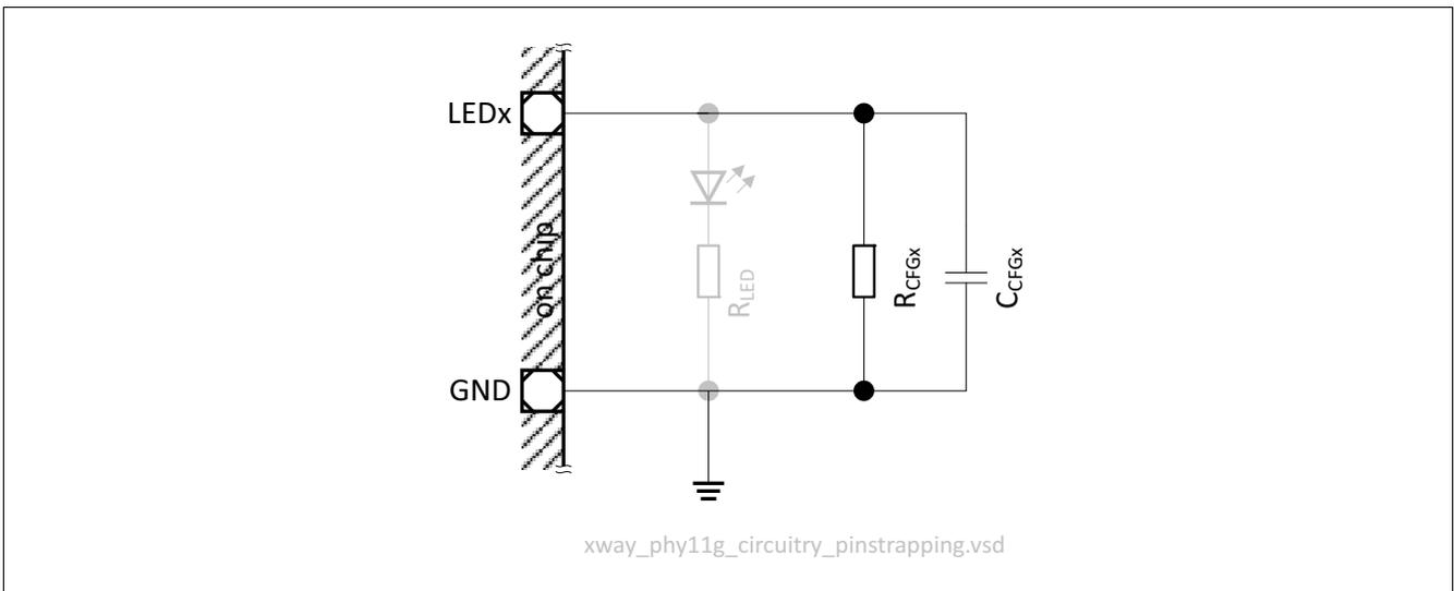
**Figure 13** Soft Pin-Strapping External Circuitry
