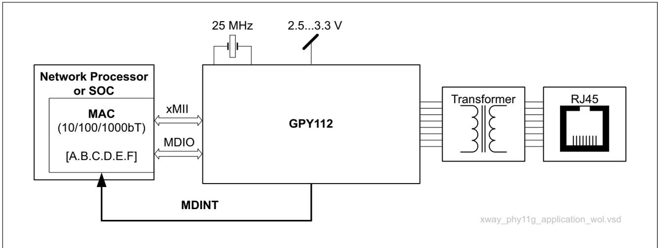
**Figure 32 Block Diagram of a WoL Application**
