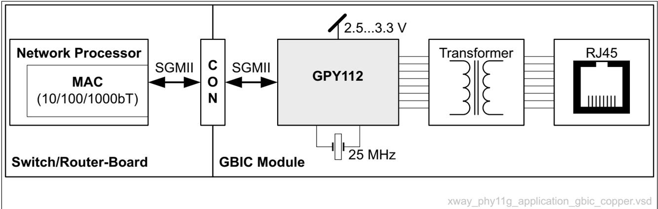
Figure 6 GPY112 Used in 10/100/1000BASE-T GBIC Application
