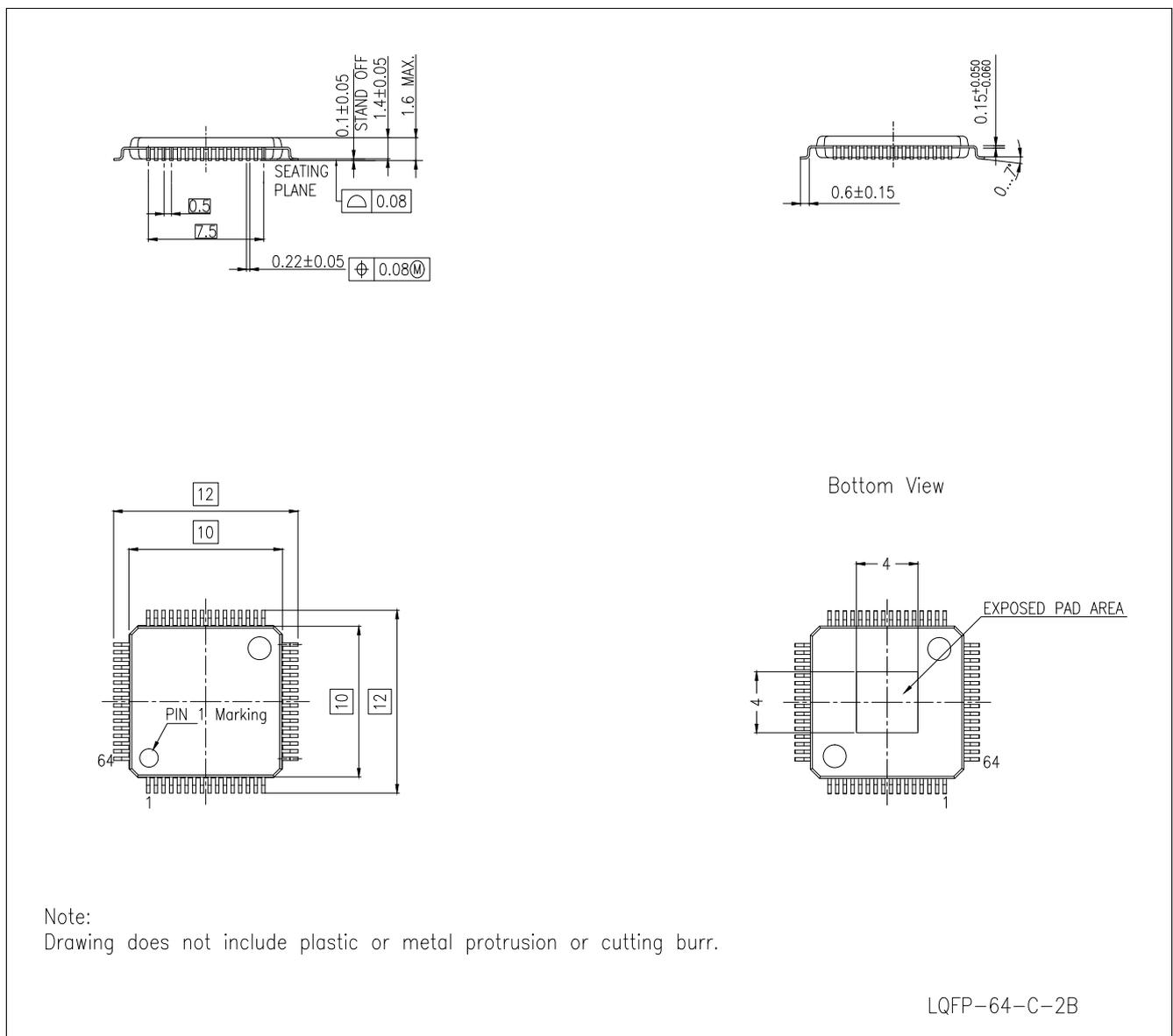
Figure 61 Package Outline Drawing of the PG-LQFP-64 Package
