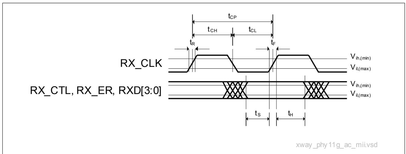
**Figure 43 Receive Timing Diagram of the MII**
