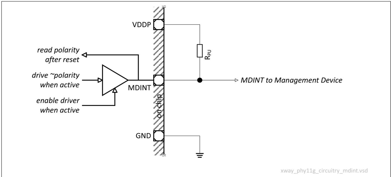
Figure 26 External Circuitry for an Active-Low MDINT
