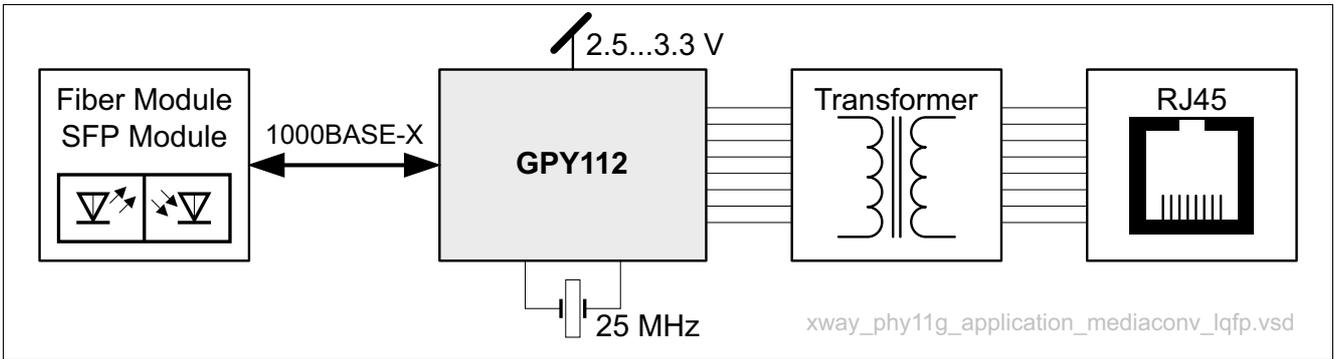
Figure 4 GPY112 Used in Media Converter Applications
