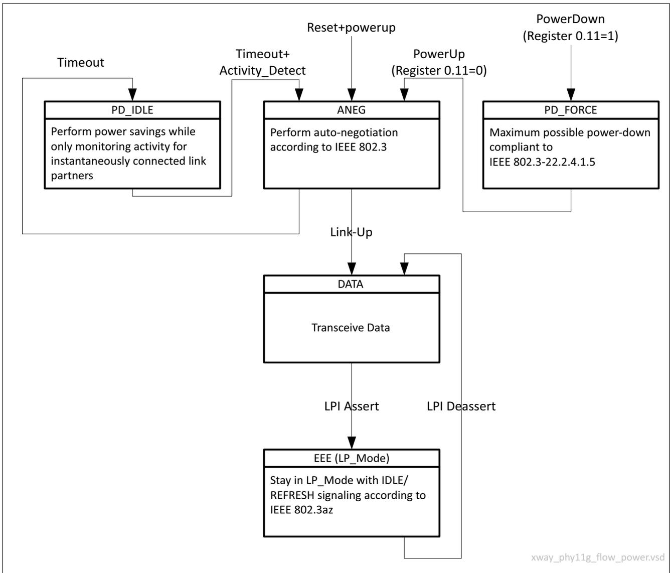
Figure 34 State Diagram for Power-Down Mode Management
