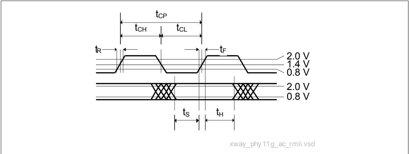
Figure 44 Transmit/Receive Timing Diagram of the RMII
