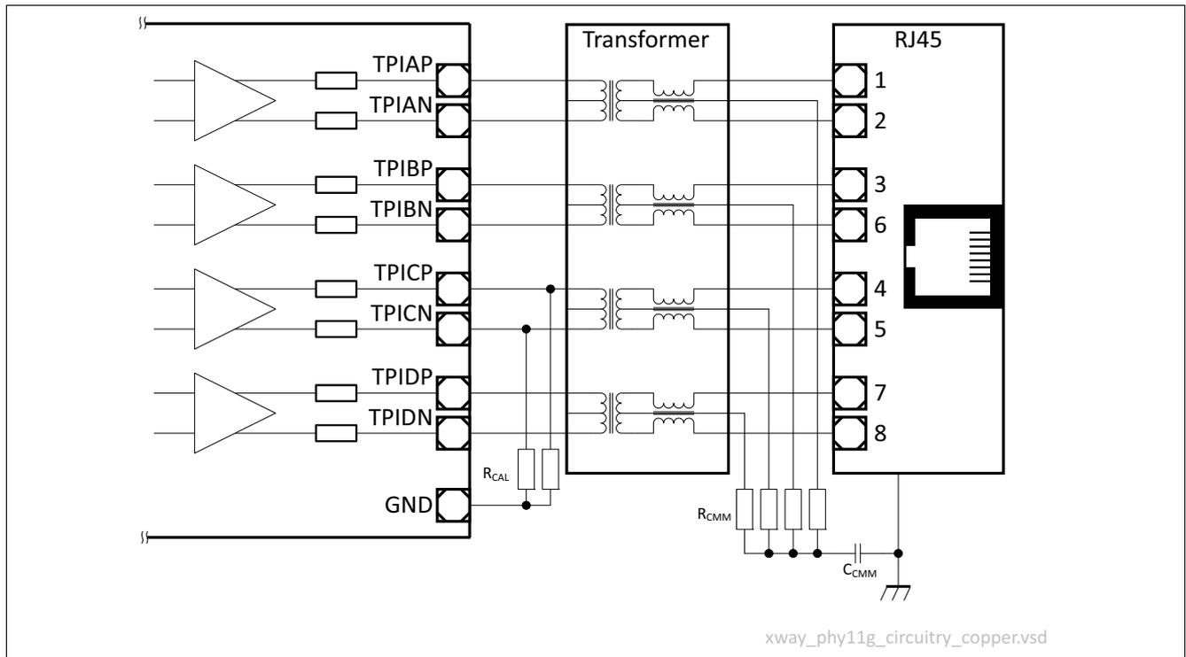
**Figure 56 Twisted-Pair Common-Mode Rejection and Termination Circuitry**
