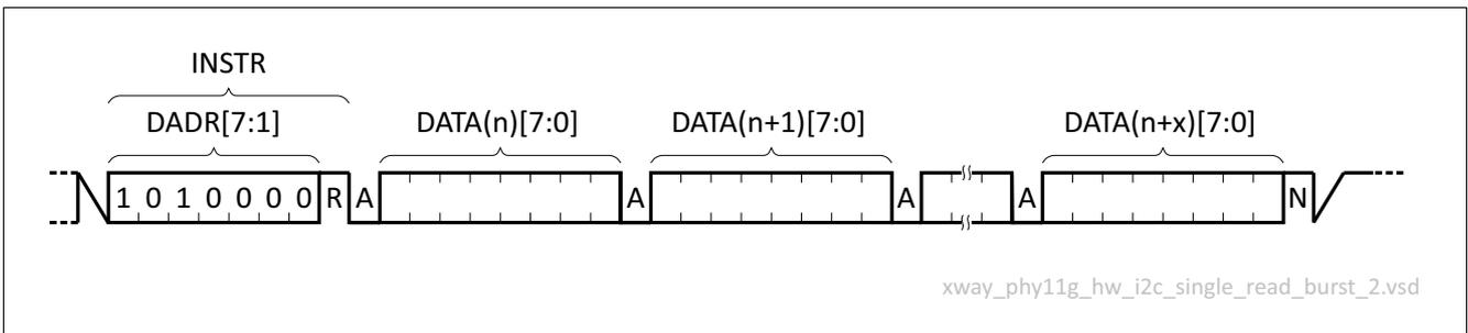
Figure 19 Timing Diagram for a Burst Read
