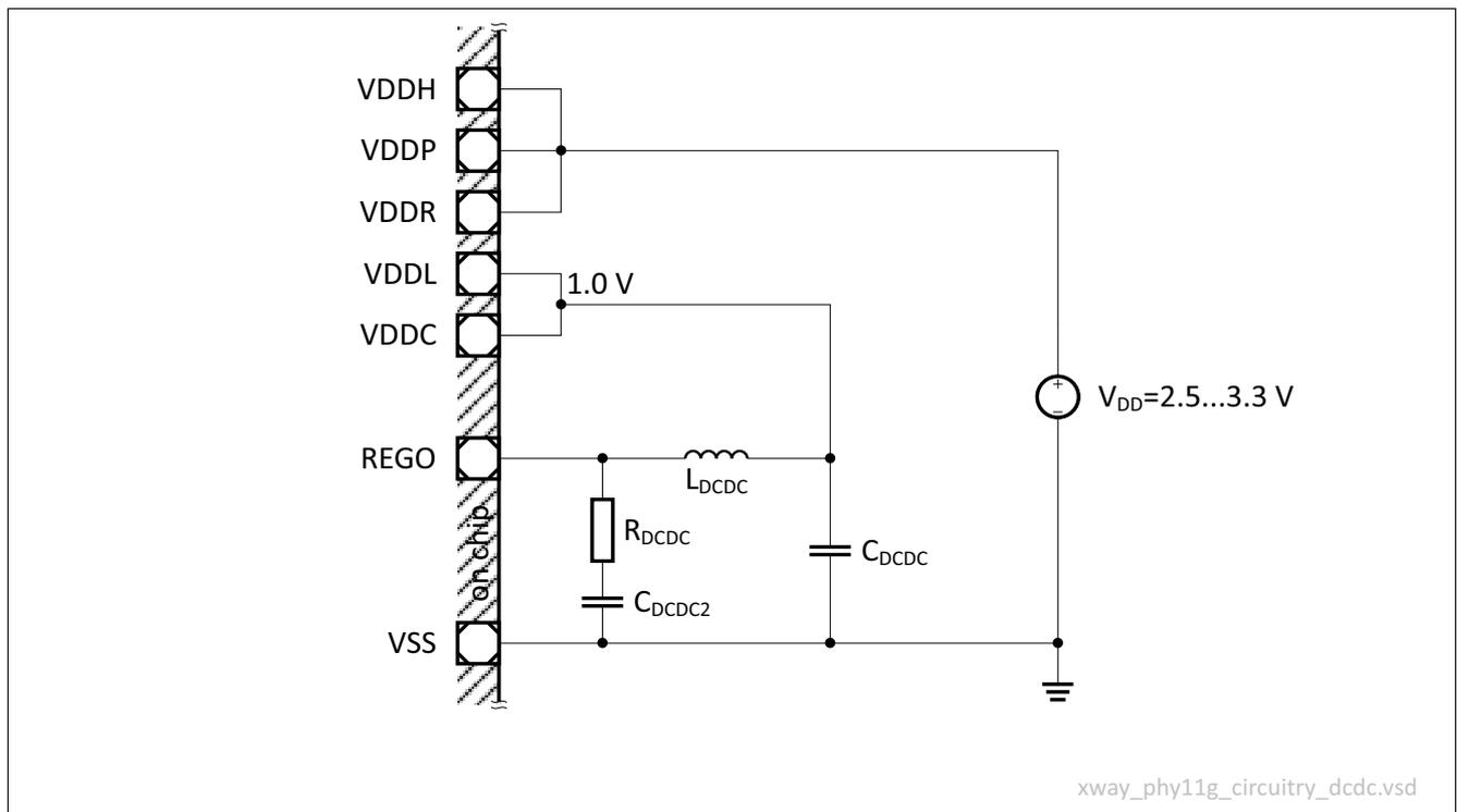
**Figure 29 External Circuitry using the Integrated Switching Regulator**
