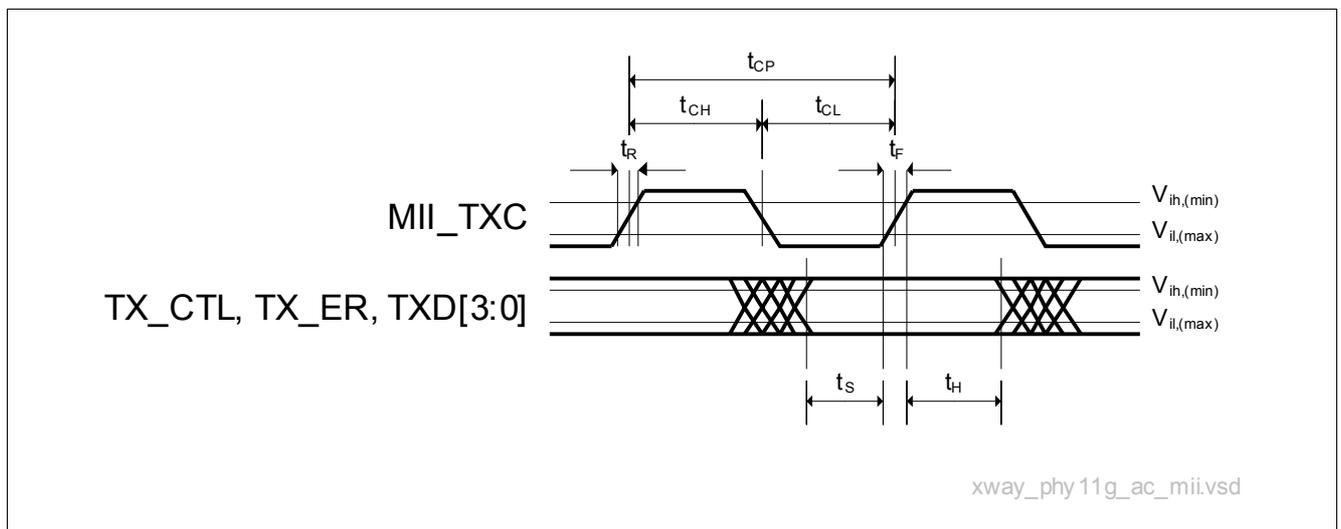
**Figure 42 Transmit Timing Diagram of the MII**
