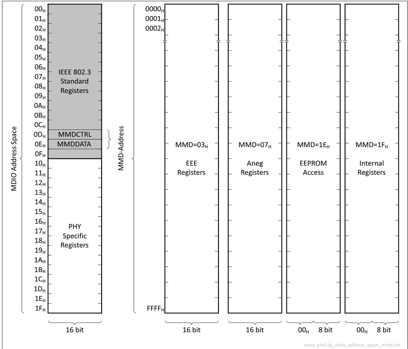
Figure 24 Layout of the MDIO Address Space
