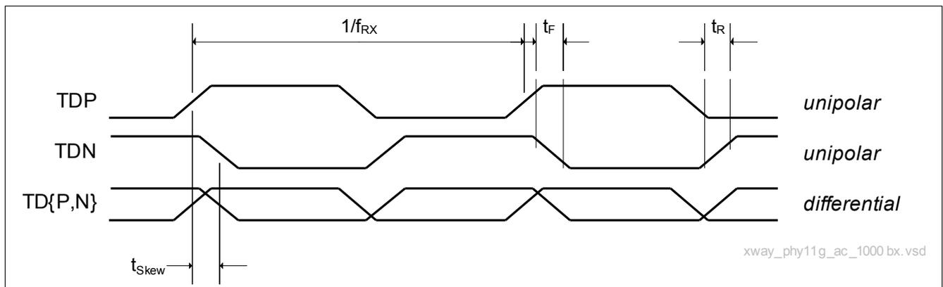
**Figure 51** Transmit Timing Diagram of the 1000BASE-X Interface
