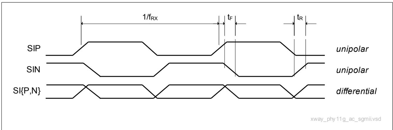
Figure 50 Receive Timing Diagram of the SGMII
