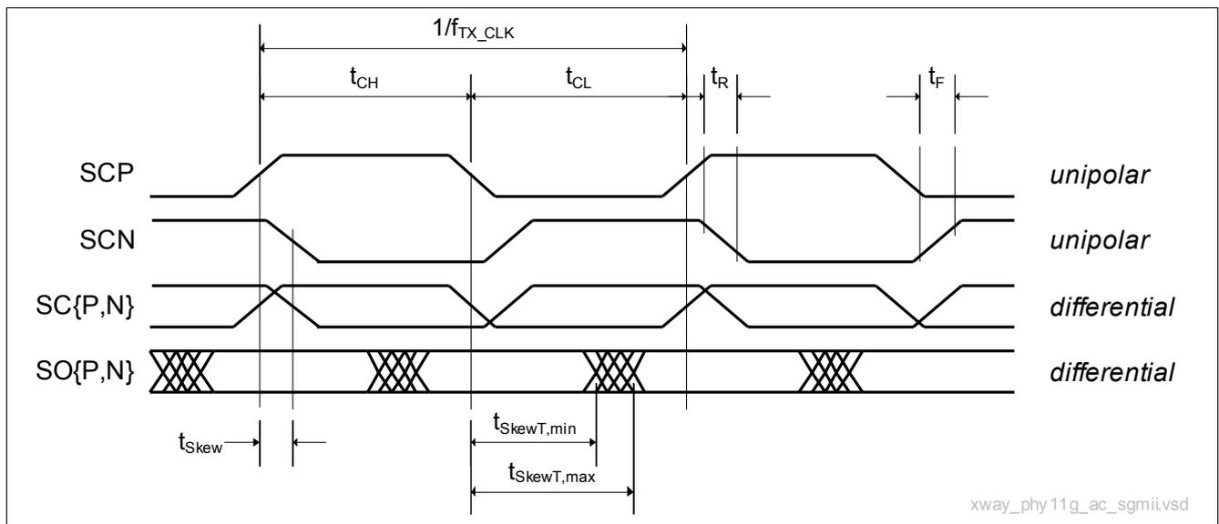
Figure 49 Transmit Timing Diagram of the SGMII
