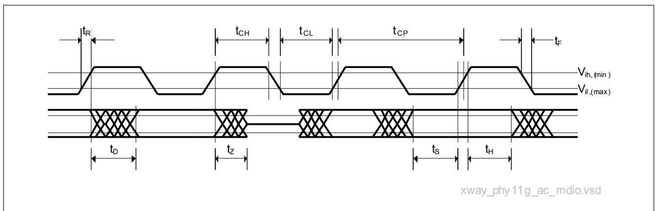
**Figure 41 Timing Diagram for the MDIO Interface**
