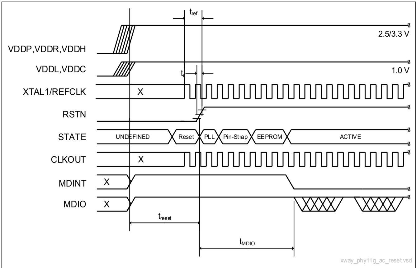
**Figure 40** Timing Diagram for the GPY112 Reset Sequence
