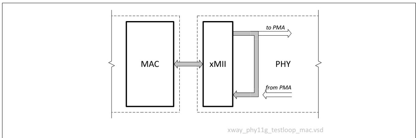
Figure 36 MAC Interface Near-End Test Loop
