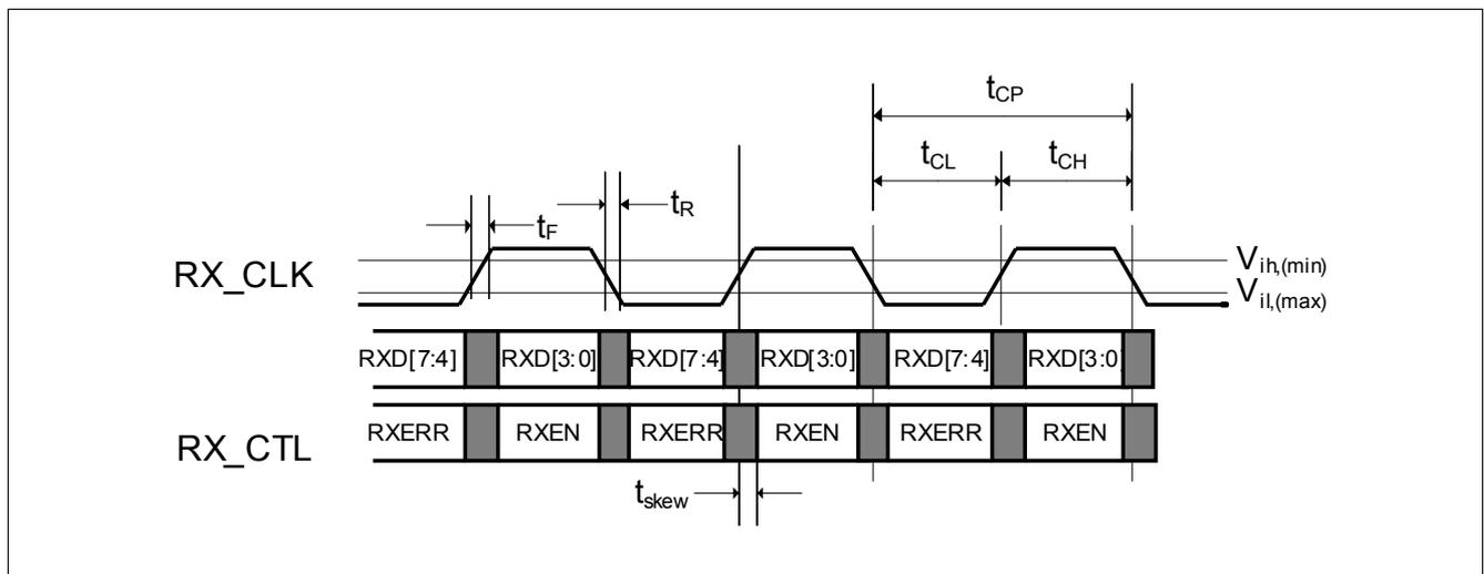
**Figure 48 Receive Timing Diagram of the RGMII**
