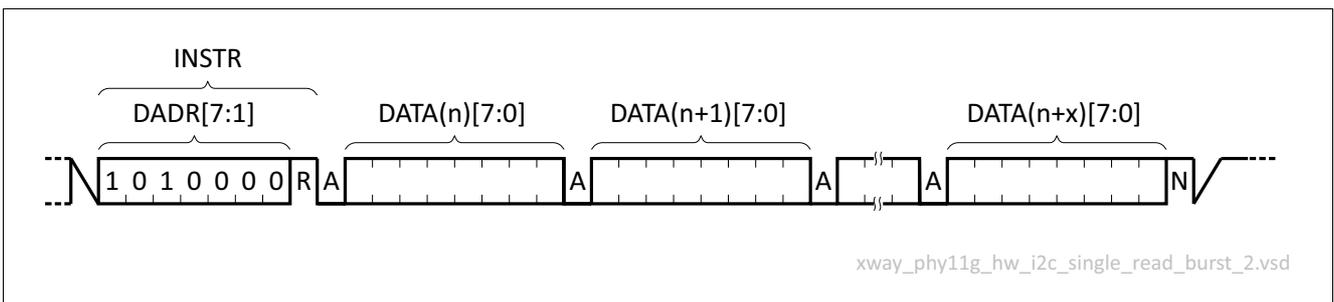
**Figure 16 Timing Diagram for a Burst Read**
