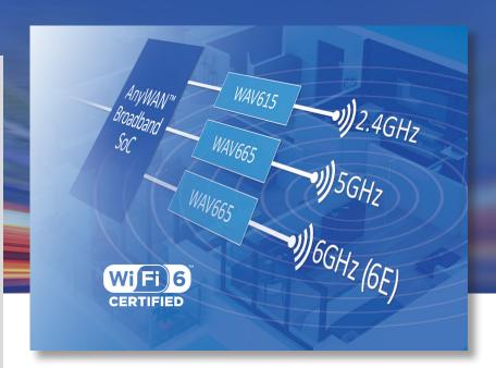
MaxLinear's 6th Generation Wi-Fi Chipset Series-2 delivers on the major features of the 802.11ax standard which further increases the reach, network capacity per user, and battery life of connected client devices. The Wi-Fi 6 Series-2 chipset is designed to deliver both fast and consistent connectivity in home Wi-Fi routers, gateways, and intelligent range extenders for cable, xDSL, fiber, and consumer retail infrastructure.
