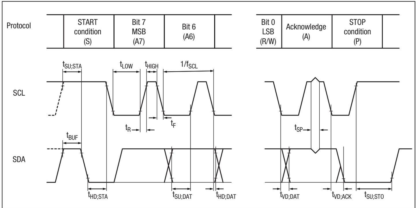
**Figure 1: I<sup>2</sup>C Bus Timing Diagram**
