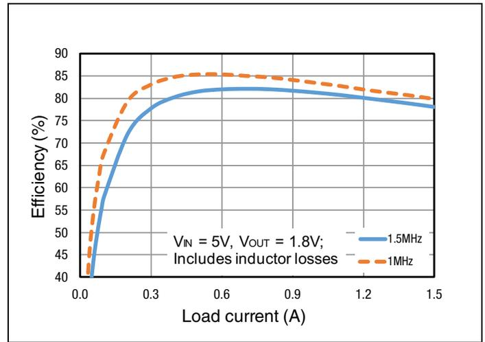
**Figure 4: Buck 2 Efficiency**
