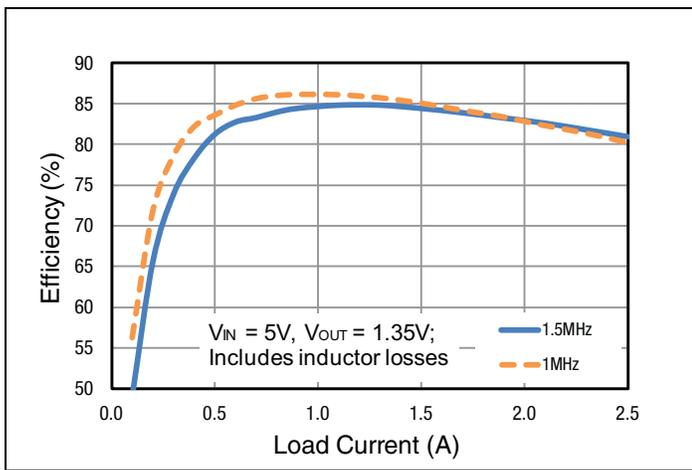
**Figure 5: Buck 3 Efficiency**
