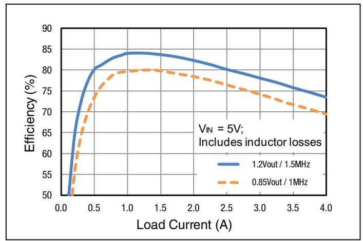
**Figure 6: Buck 4 Efficiency**
