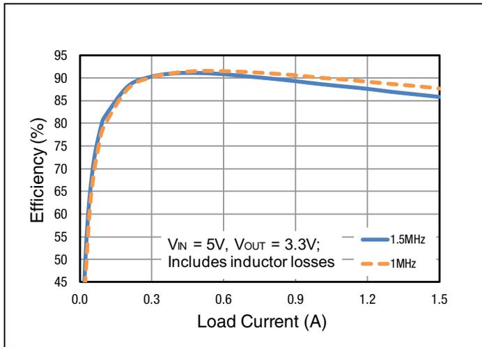
**Figure 3: Buck 1 Efficiency**
