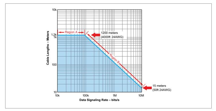
Figure 2: Cable Lengths versus Data Signaling Rate
