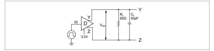
Figure 1: RS-485 Differential Output Voltages (V<sub>OD</sub>)
