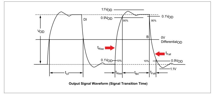
Figure 3:  $t_{Rise,} t_{Fall}$  and  $t_{UI}$  Signal Transition Time Requirements
