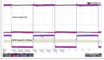
Figure 4: Eye-Diagram at Driver Output
