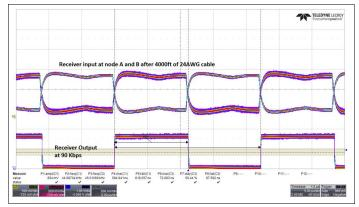
Figure 5: Eye-Diagram at Receiver Input after 4000ft Cable @90Kbps
