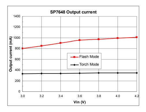
Figure 1. Output Current Regulation vs. Battery Voltage in Flash and Torch modes
