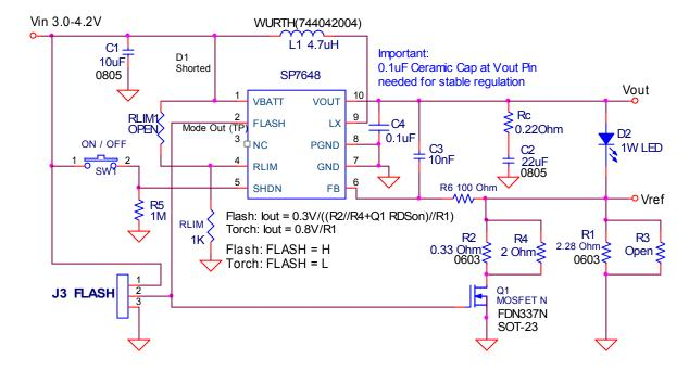
Figure 6. Applications Schematic
