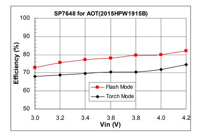
Figure 2. Boost Converter Efficiency in Flash and Torch Modes
