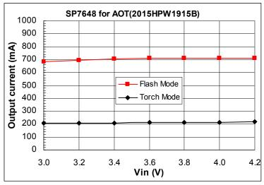
Figure 1. Output Current Regulation vs. Battery Voltage in Flash and Torch modes
