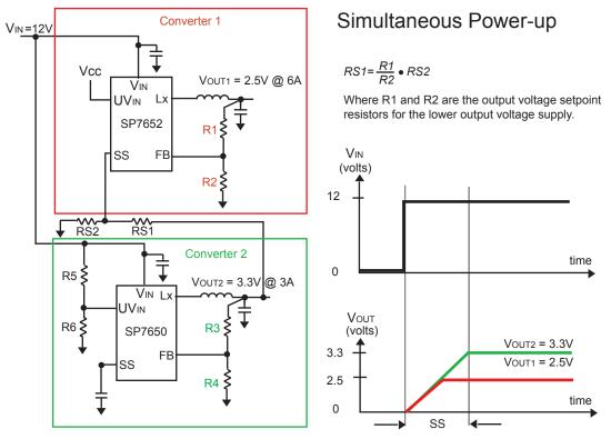
Figure 5. Simultaneous Power-up Using PowerBlox™
