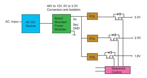
Figure 1. Distributed Power Architecture in a Telecommunications System
