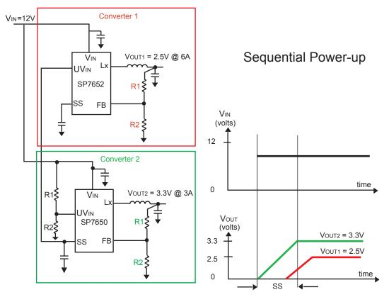
Figure 3. Sequential Power-up Implemented with PowerBlox™
