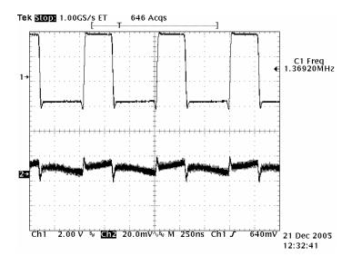
Channel 2 V<sub>out</sub> ripple Channel 1 Switch Node  $I_{out}$  500mA
