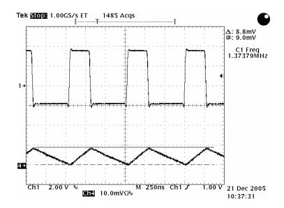
Channel 1 Switch node Channel 2 is Inductor Current  $I_{L}$   $I_{out}\,was\,50mA$  Current setting is 200mA/Div
