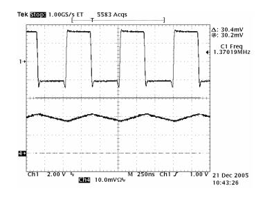
Channel 1 Switch node Channel 2 is Inductor Current  $I_{\rm L}$   $I_{out}\,was\,500mA\,Current$  setting is 500mA/Div
