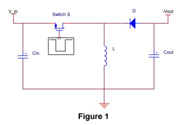
One advantage of using the SP6652 is the integration of the synchronous FET into the device, thus eliminating the need for the free wheeling diode D. This helps reduce the part count as well as increase the efficiency of the overall circuit. Below in Figure 2 is the switch configuration of the SP6652 showing how the synchronous switch Sync\_FET replaces the free wheeling diode D.
