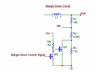
Figure 6 – Margin Down Circuit
