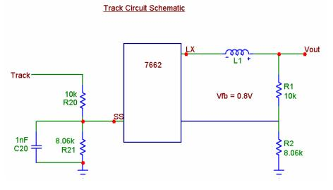
Figure 4 – Track Feature Connection diagram
