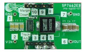
Figure 10 – Complete POLA™ part evaluation board
