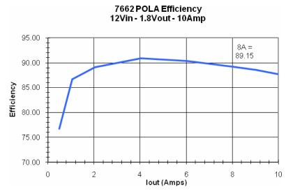
Figure 8 – Design Efficiency (POLA<sup>™</sup> quoted efficiency at 8Amp = 87%)
