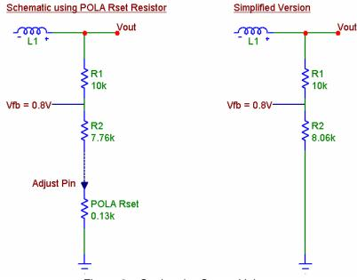
Figure 2 – Setting the Output Voltage
