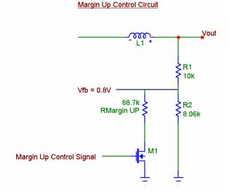
Figure 5 – Margin Up Resistor Connection
