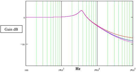
Diagram 6 gain of boost regulator with load resistance variations Red RL is 5 ohms Blue RL is 10 ohms Magenta RL is 15 ohms
