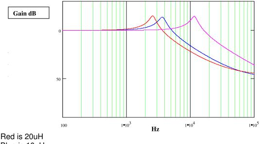
Red is 20uH Blue is 10uH Magenta is 1uH Diagram 8 Example of different inductor values on the boost regulator filter
