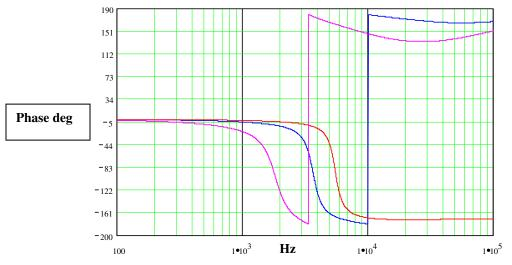
Diagram 5 Bode Plot Boost Regulator Phase for different duty cycle Magenta Duty cycle of .75 Blue Duty cycle of .5 Red Duty cycle of .25
