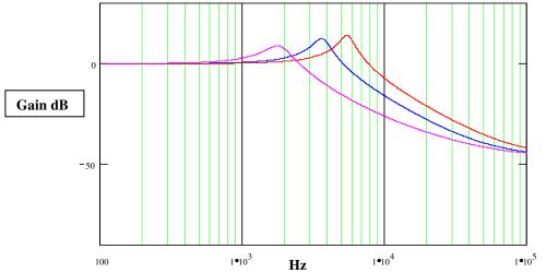
Diagram 4 Bode Plot Boost regulator Gain for different duty cycle Magenta Duty cycle of .75
