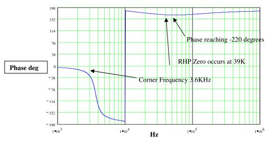
Diagram 3 Phase of a boost regulator in diagram 1 duty cycle=.5
