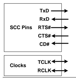
The signal names and directions reflect their function in a DTE configuration, but an SCC may be programmed to operate as either DTE or DCE.
