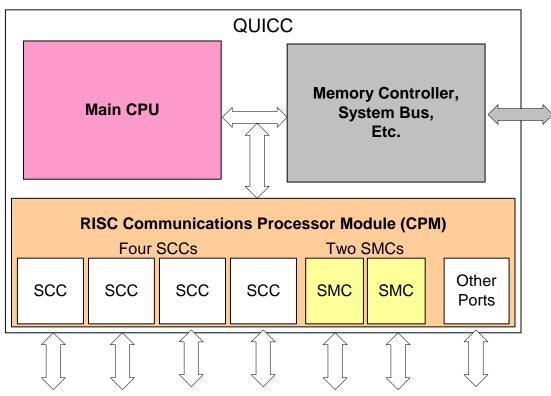
QUICC<sup>™</sup> Architecture - Simplified Block Diagram
