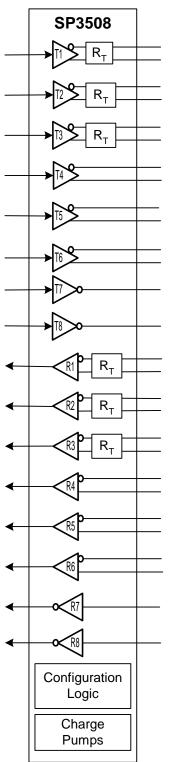
The SP3508, SP508 and SP509 are all highly integrated multiprotocol serial transceivers. Each have a total of 8 drivers and 8 receivers and can be configured to support a variety of standard serial port standards.
