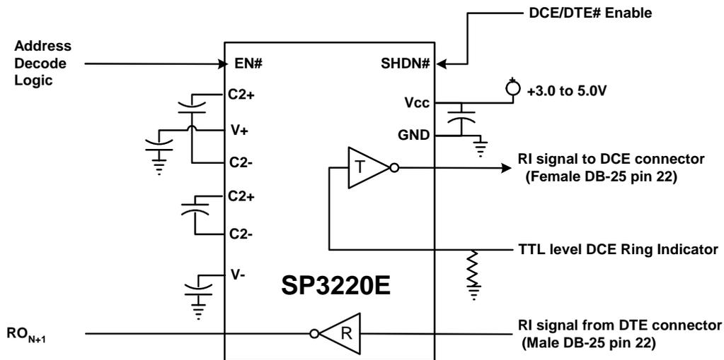
Some protocols such as RS-232 and RS-449 allow for secondary data channels and also include a number of other diagnostic signals. Use of these additional channels and signals is rare. But if they are required they must be implemented using additional external transceivers.
