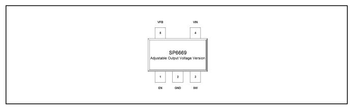
Fig. 2: SP6669 Pin Assignment
