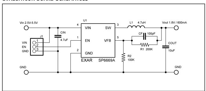
Fig. 1: SP6669 Evaluation Board Schematics
