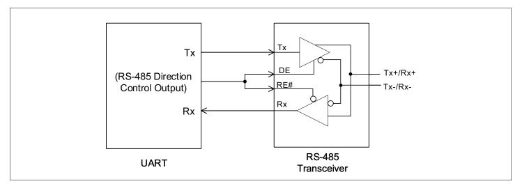
Figure 1: Typical Connection between UART and RS-485 Transceiver
