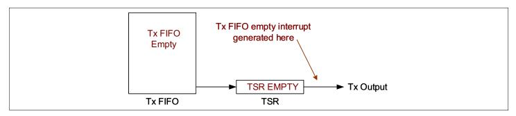
Figure 3: UART Transmit Interrupt Behavior with Auto RS-485 Feature
