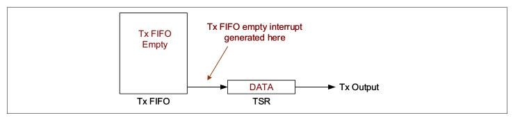
Figure 2: UART Transmit Interrupt Behavior
