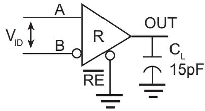
Receiver DC Test Circuit
