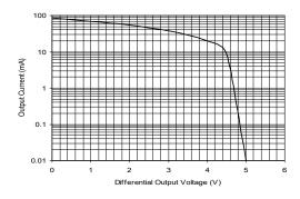
Driver Output Current vs Differential Output Voltage
