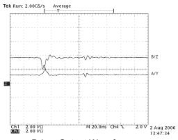
Driver Output Waveforms High to Low
