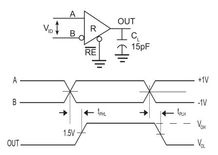
Receiver Propagation Delay Test Circuit and Timing Diagram
