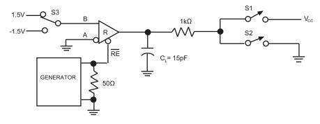
Receiver Enable and Disable Times Test Circuit
