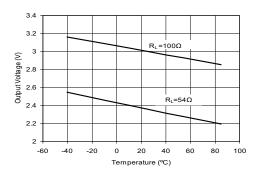
Driver Differential Output Voltage vs Temperature
