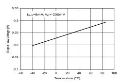
Receiver Output Low Voltage vs Temperature
