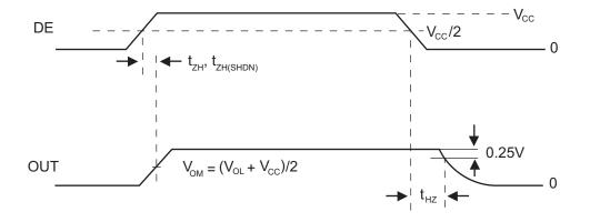
Driver Enable and Disable Times Test Circuit and Timing Diagram
