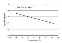
Receiver Output High Voltage vs Temperature
