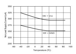
No-load Supply Current vs Temperature
