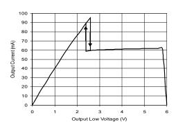
Output Current vs Driver Output Low Voltage
