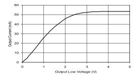
Output Current vs Receiver Output Low Voltage
