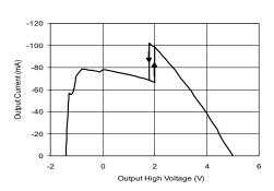
Output Current vs Driver Output High Voltage
