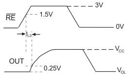
Receiver Enable and DisableTiming Diagram
