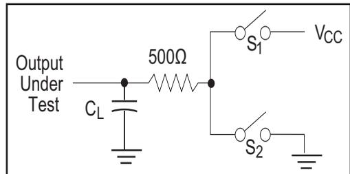
Figure 5. Driver Timing Test Load #2 Circuit
