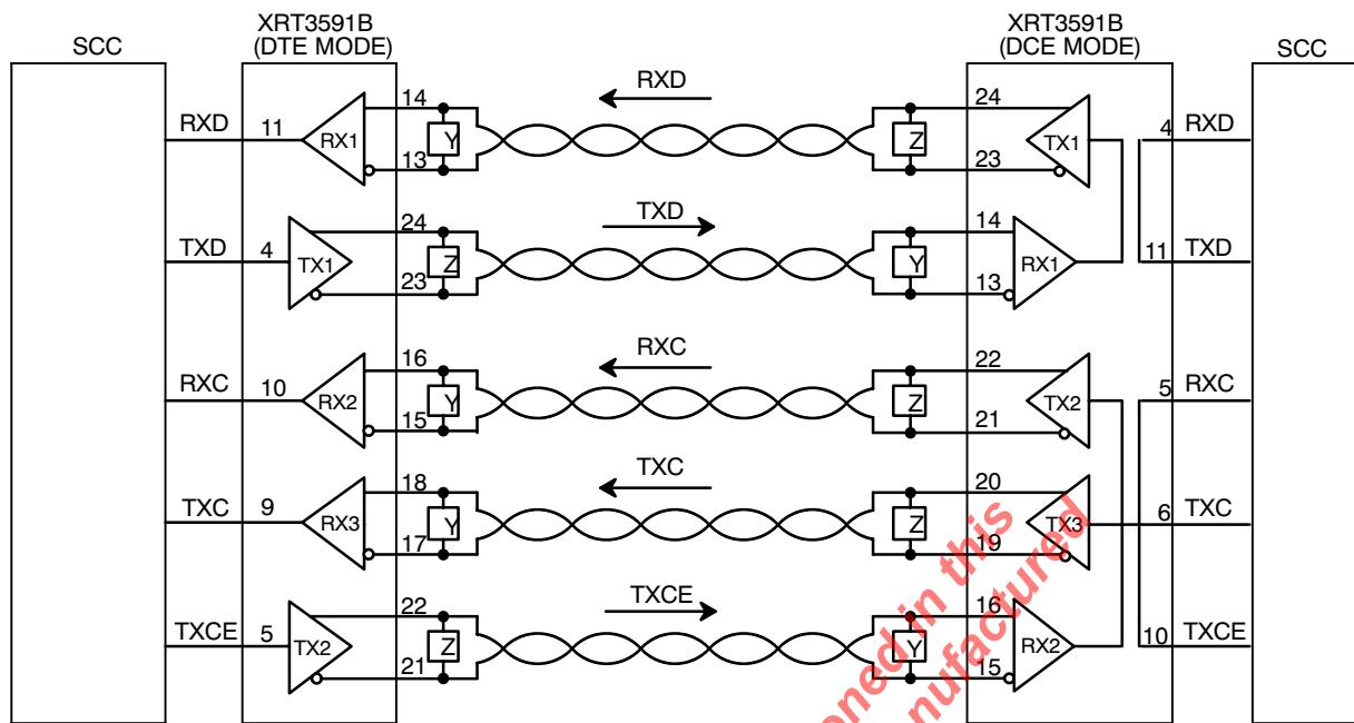
Figure 7. Typical V.35 Configuration During DCE Mirrored Loopback
