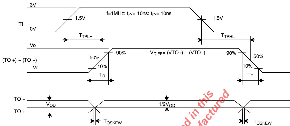
Figure 3. V.35 Transmitter Propagation Delays
