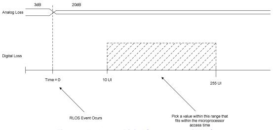
Figure 1. Analog and Digital Components of RLOS
