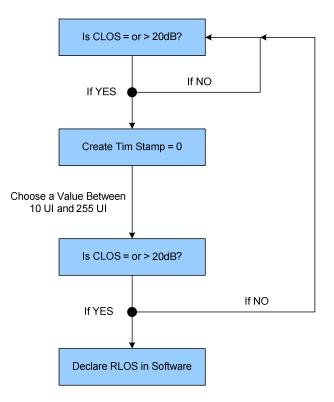
Figure 2. Flow Chart of a Typical Software Routine for RLOS
