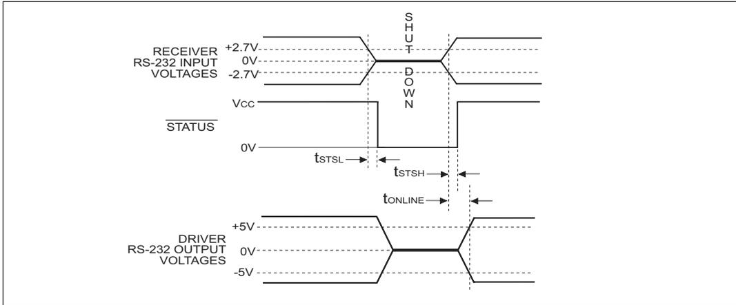
Figure 13. AUTO ON-LINE<sup>®</sup> Timing Waveforms
