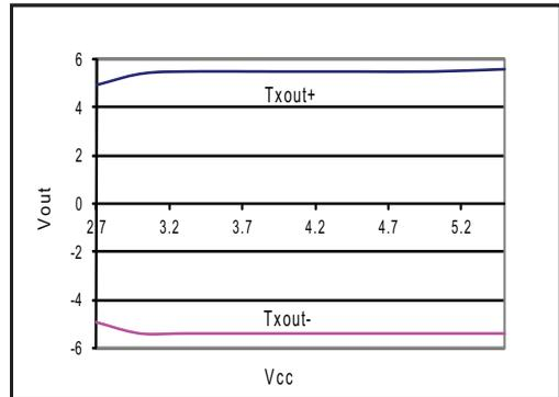
Figure 3. Transmitter Output Voltage VS. Supply Voltage
