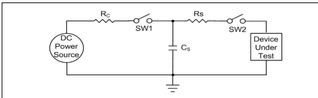
Figure15. ESD Test Circuit for Human Body Model
