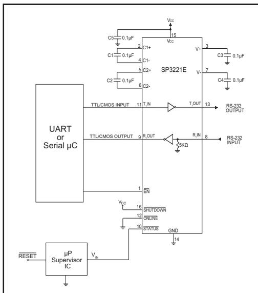
Figure 5. Interface Circuitry Controlled by Microprocessor Supervisory Circuit (\*)
