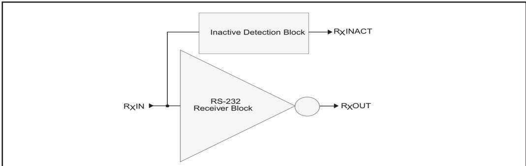
Figure 14. Stage I of AUTO ON-LINE<sup>®</sup> Circuitry
