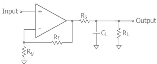
Figure 4. Addition of  $R_S$  for Driving Capacitive Loads
