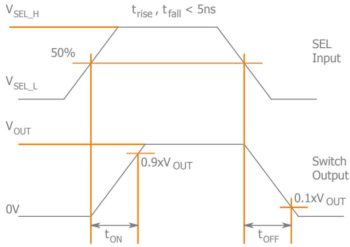
Figure 1.  $t_{ON}$ ,  $t_{OFF}$
