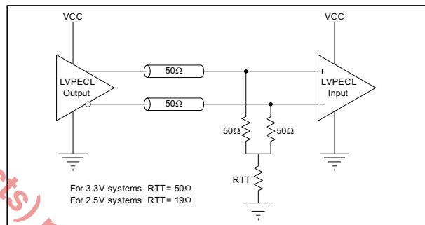
**Figure 7: XR81111 Alternate LVPECL Output Termination Using Y-termination**
