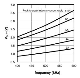
Figure 12:  $V_{OUT}$  versus f,  $V_{IN}$ =12V
