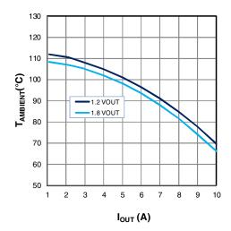
Figure 24: Maximum T<sub>AMBIENT</sub> vs I<sub>OUT</sub>, V<sub>IN</sub>=19.6V
