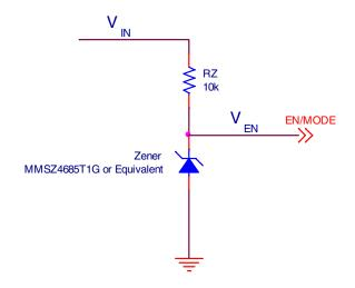
Figure 26: Selecting DCM/CCM by deriving EN/MODE from V<sub>IN</sub>
