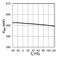
Figure 8: V<sub>REF</sub> versus temperature
