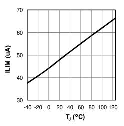
Figure 9: I<sub>LIM</sub> versus temperature
