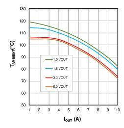
Figure 22: Maximum  $T_{AMBIENT}$  vs  $I_{OUT}$ ,  $V_{IN}$ =12V
