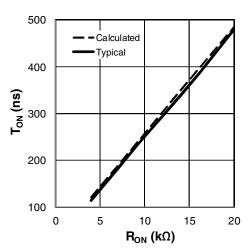
Figure 3: T<sub>ON</sub> versus R<sub>ON</sub>
