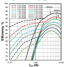
Figure 21: Efficiency, V<sub>IN</sub>=12V
