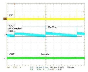
Figure 14: Steady state, DCM, I<sub>OUT</sub>=0A
