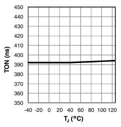
Figure 10:  $T_{ON}$  versus temperature,  $R_{ON}$ =16.2 $k\Omega$
