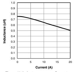
Figure 11: Inductance versus Current
