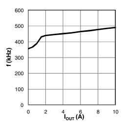
Figure 5: frequency versus I<sub>OUT</sub>
