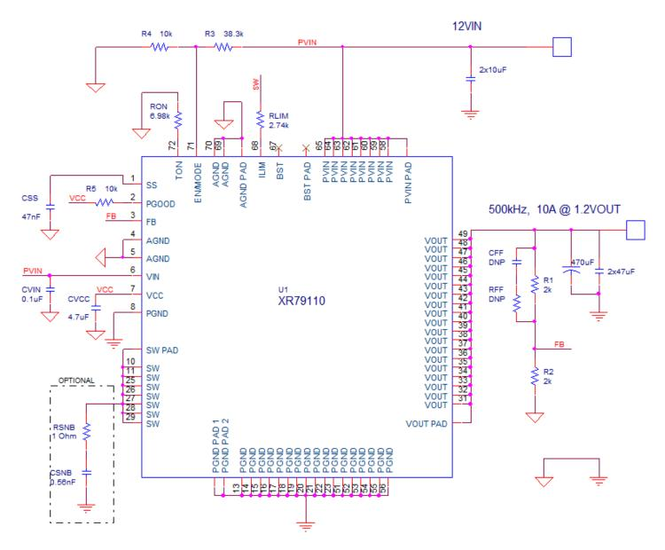
Note 1: Snubber circuit to be used when large transients on SW node.
