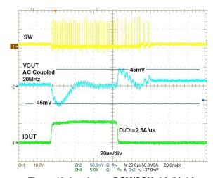
Figure 18: Load step, DCM/CCM, 0A-5A-0A
