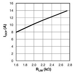
Figure 7: I<sub>OCP</sub> versus R<sub>LIM</sub>
