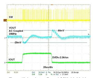
Figure 17: Load step, Forced CCM, 0A-5A-0A
