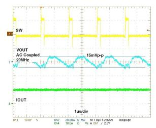
Figure 13: Steady state, CCM, I<sub>OUT</sub>=10A
