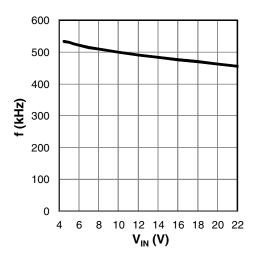
Figure 6: frequency versus V<sub>IN</sub>
