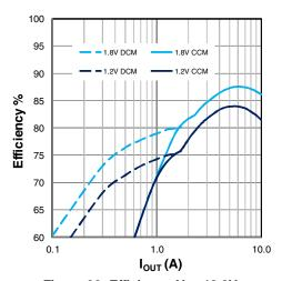
Figure 23: Efficiency, V<sub>IN</sub>=19.6V
