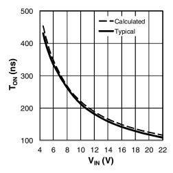
Figure 4: T<sub>ON</sub> versus V<sub>IN</sub>, R<sub>ON</sub>=6.98k
