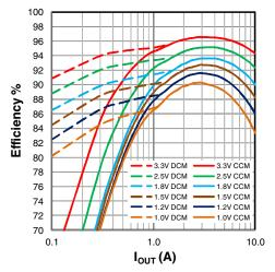
Figure 19: Efficiency, V<sub>IN</sub>=5V
