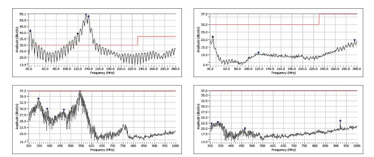
Figure 4. EMI Test Without Input/Output Filters
