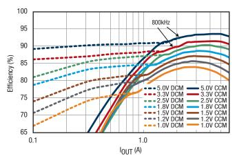
Figure 22. Efficiency, V<sub>IN</sub> = 12V
