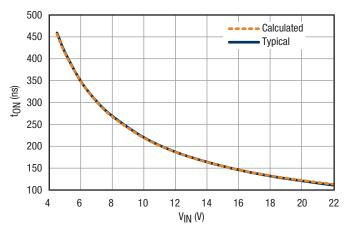
Figure 6.  $t_{ON}$  vs.  $V_{IN}$ ,  $R_{ON} = 6.98 k\Omega$
