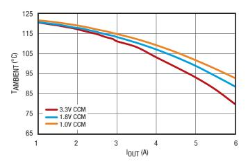
Figure 21. Maximum  $T_{AMBIENT}$  vs.  $I_{OUT}$ ,  $V_{IN} = 5V$
