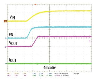
Figure 17. Power Up,  $I_{OUT} = 0A$
