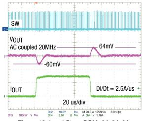
Figure 18. Load Step, CCM, 0A-3A-0A
