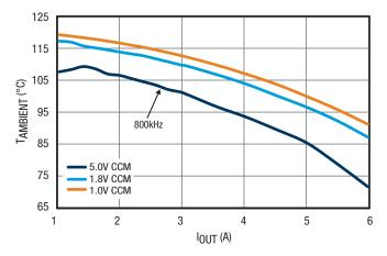
Figure 23. Maximum  $T_{AMBIENT}$  vs.  $I_{OUT}$ ,  $V_{IN} = 12V$
