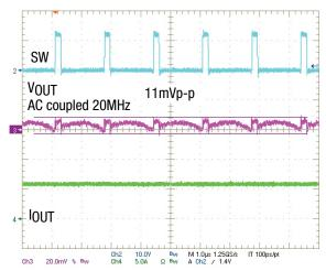
Figure 14. Steady State CCM, I<sub>OUT</sub> = 6A
