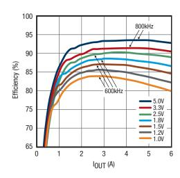
Figure 2. Efficiency, 12V<sub>IN</sub>
