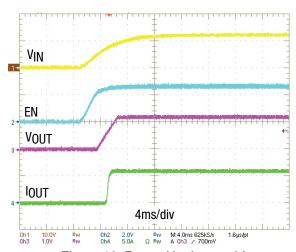
Figure 16. Power Up,  $I_{OUT} = 6A$
