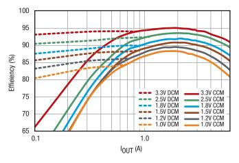
Figure 20. Efficiency, V<sub>IN</sub> = 5V
