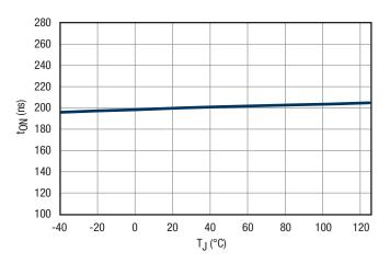
Figure 11.  $t_{ON}$  vs. Temperature,  $R_{ON} = 6.98k\Omega$
