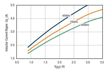
Figure 13. Inductor Current Ripple vs.  $V_{OUT}$
