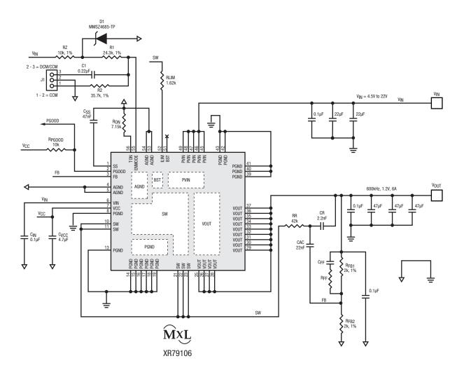
Figure 27. Typical Application Circuit
