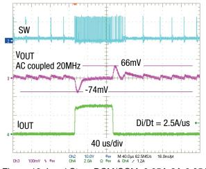
Figure 19. Load Step, DCM/CCM, 0.05A-3A-0.05A
