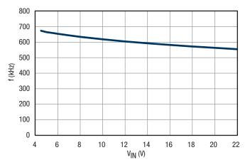
Figure 8. Switching Frequency vs. V<sub>IN</sub>
