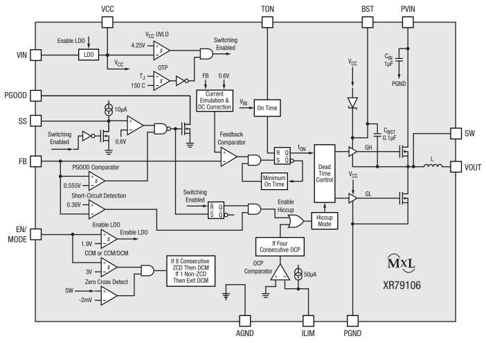
Figure 24. Functional Block Diagram
