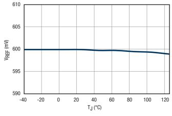
Figure 10. V<sub>REF</sub> vs. Temperature
