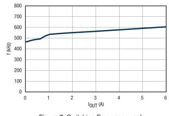
Figure 7. Switching Frequency vs.  $I_{OUT}$
