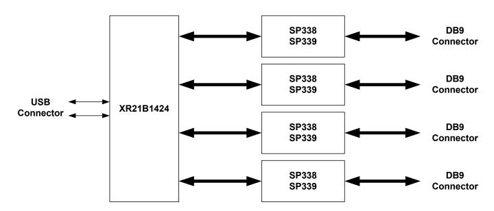
Figure 1: Evaluation Board Block Diagram
