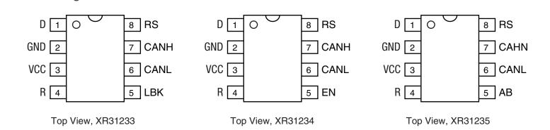
Figure 3: Pin Configurations for the XR31233, XR31234 and XR31235 CAN Bus Transceivers
