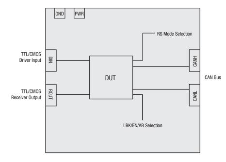
Figure 2: Block Diagram XR31233 / XR31234 / XR31235 - EVB
