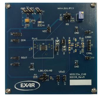
Figure 1: Top View of XR31233 / XR31234 / XR31235 EVB
