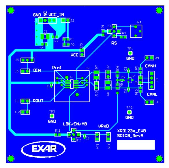
Figure 5: XR31233 / XR31234 / XR31235 EVB, Top View
