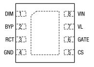
3mm x 3mm DFN-8L, Top View
