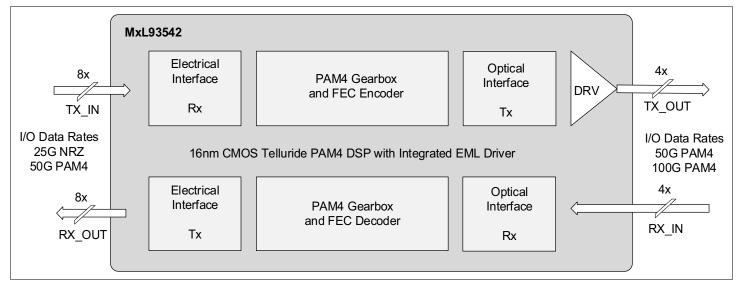
Figure 1: MxL93542 Functional Block Diagram
