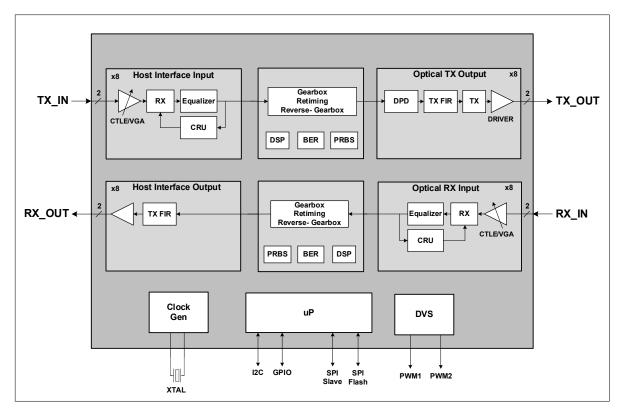
Figure 1: MxL9368x Simplified Block Diagram
