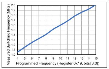
Figure 8: Measured vs Programmed Frequency
