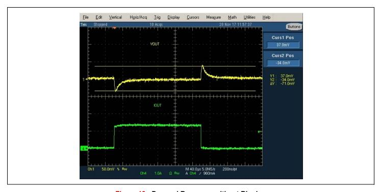
Figure 18: Damped Response without Ringing
