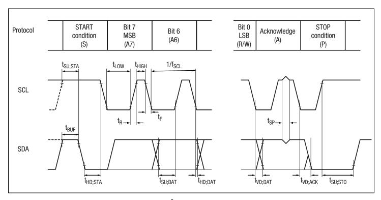
Figure 1: I<sup>2</sup>C Bus Timing Diagram
