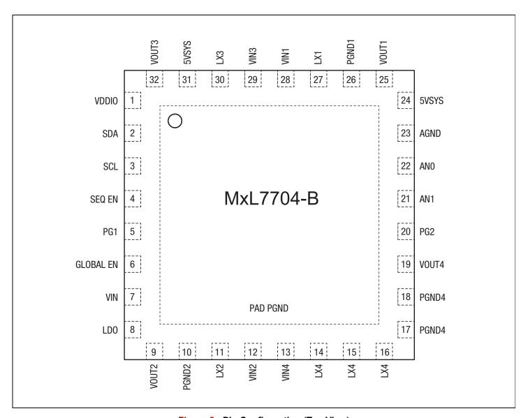
Figure 2: Pin Configuration (Top View)
