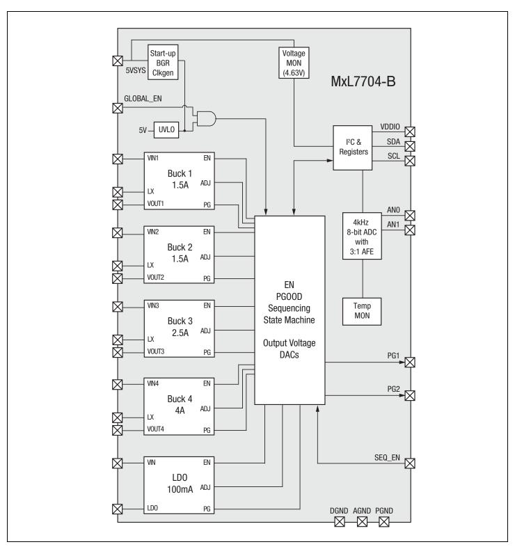
Figure 14: Functional Block Diagram
