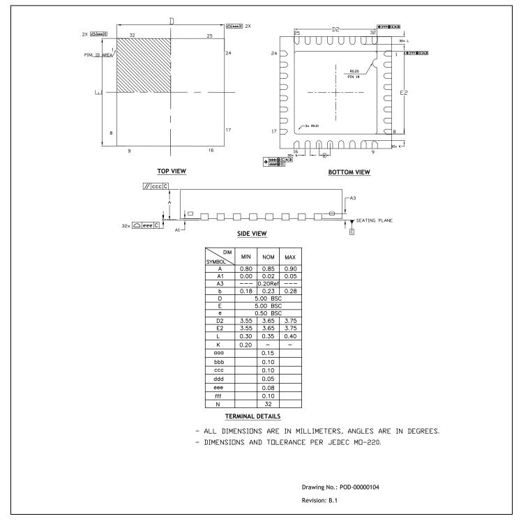
Figure 20: Mechanical Dimensions
