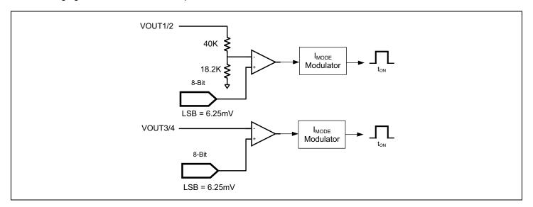
Figure 17: MxL7704-B Control Loop Architecture
