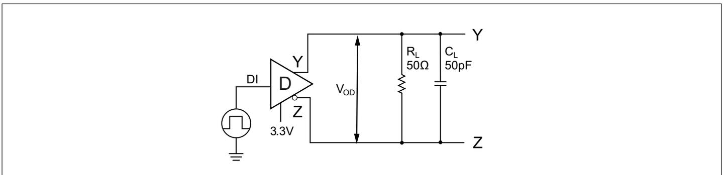
**Figure 1: RS-485 Differential Output Voltages ( $V_{OD}$ )**
