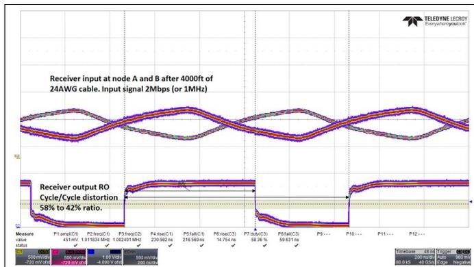
**Figure 6: Eye-Diagram at Receiver Input after 4000ft Cable @2Mbps**
