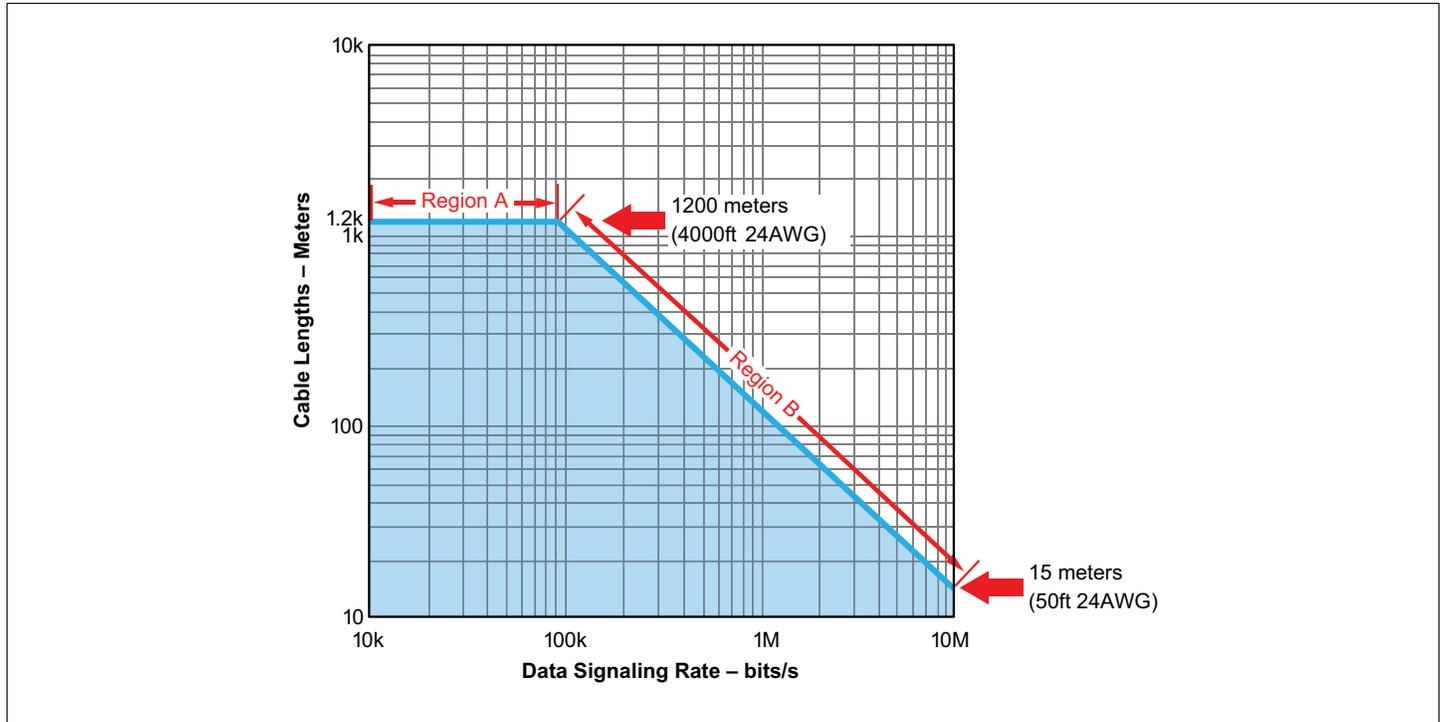
**Figure 2: Cable Lengths versus Data Signaling Rate**
