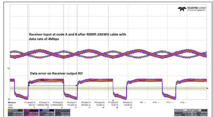
**Figure 7: Eye-Diagram at Receiver Input after 4000ft Cable @4Mbps**
