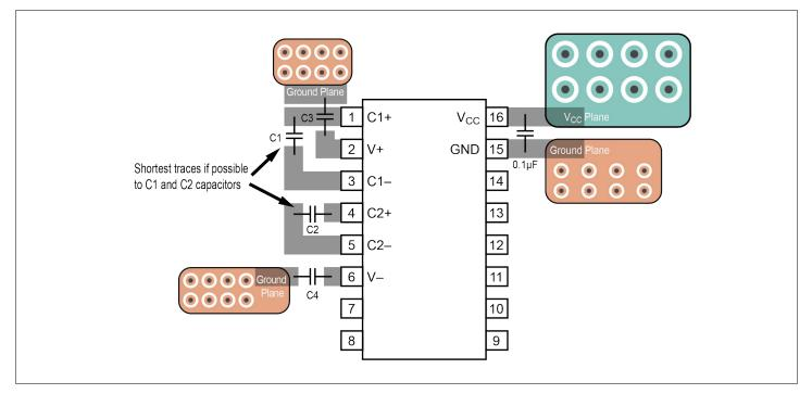
Figure 2: Optimal Use of Power Supply Traces, Ground Planes, and Power Planes
