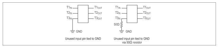
Figure 3: Input Traces and Unused Input Pin Strapping Recommendation
