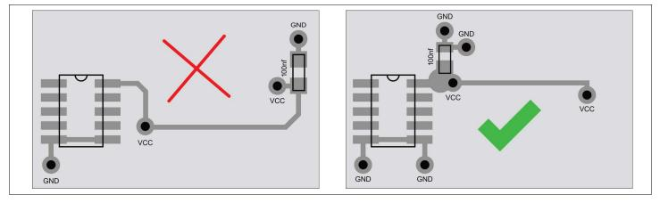
Figure 1: Optimal Power Supply Decoupling Capacitor Location
