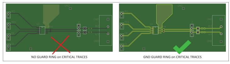
Figure 5: Example of a Guard Ring around Critical Traces
