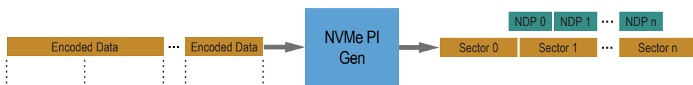
Figure 10: NVMe PI Fields Generated and Returned in Sideband Buffer as a DIX-Style NVMe PI
