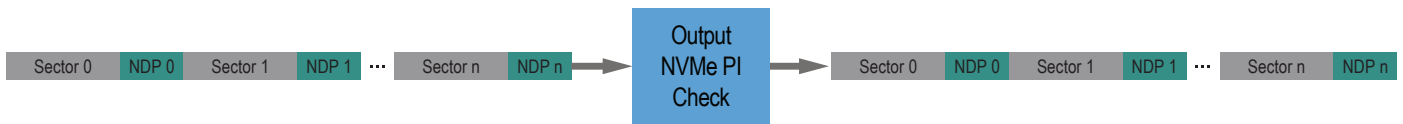
Figure 13: Decoded Data has NVMe PI Fields Verified and Returned as Embedded Fields in the Decoded Data
