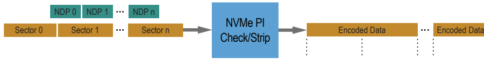
Figure 11: Encoded Data for Decode has NVMe PI Fields Supplied in Sideband Buffer in DIX Style to be Verified and Discarded
