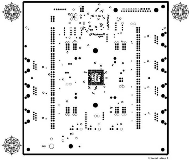
**Figure 11 XRT83SL38/L38EVAL BGA Layout Plot-Ground Plane**
