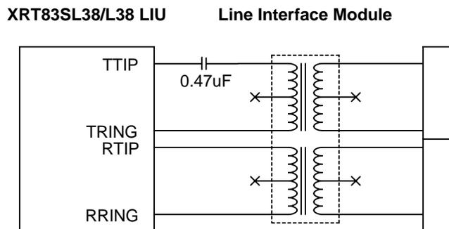
**Figure 3 Simplified Block Diagram of the Internal Impedance Mode**
