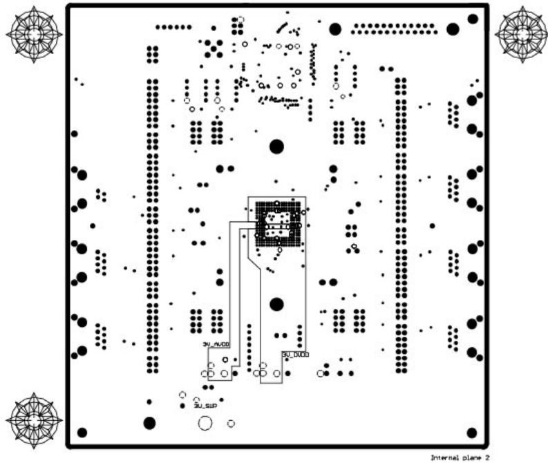
**Figure 12 XRT83SL38/L38EVAL BGA Layout Plot-Power Plane**
