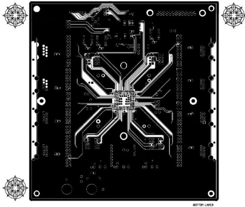
**Figure 13 XRT83SL38/L38EVAL BGA Layout Plot-Bottom Layer**
