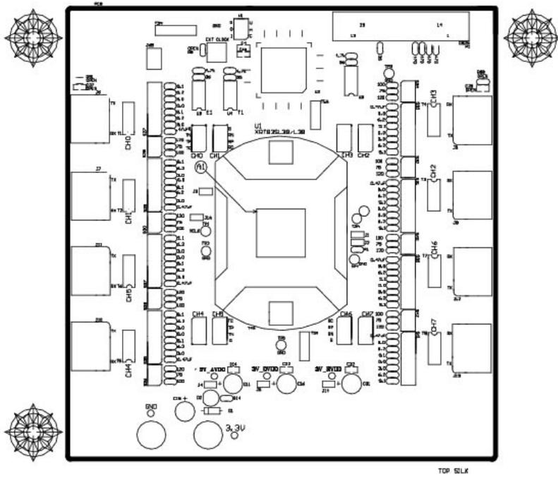
**Figure 9 XRT83SL38/L38EVAL BGA Layout Plot-Top Silk Screen**
