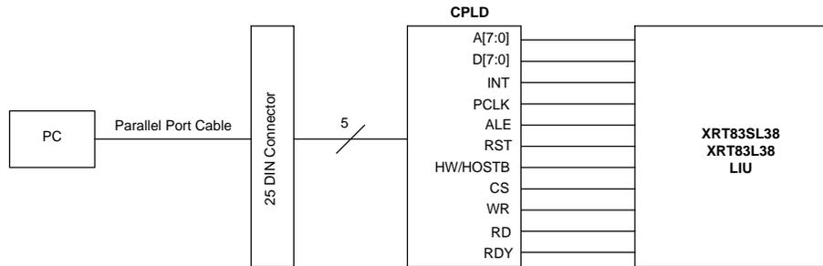
**Figure 2 Simplified Block Diagram of the CPLD Interface**
