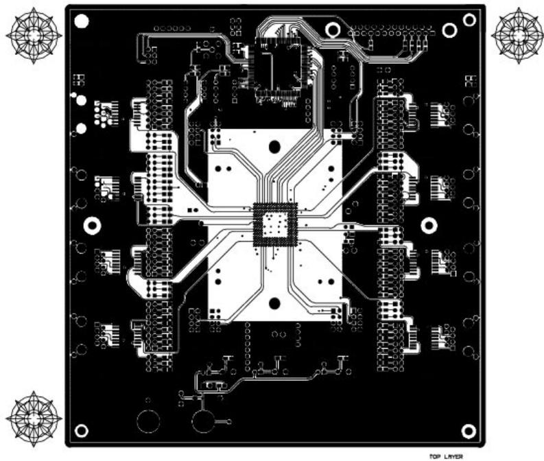
**Figure 10 XRT83SL38/L38EVAL BGA Layout Plot-Top Layer**
