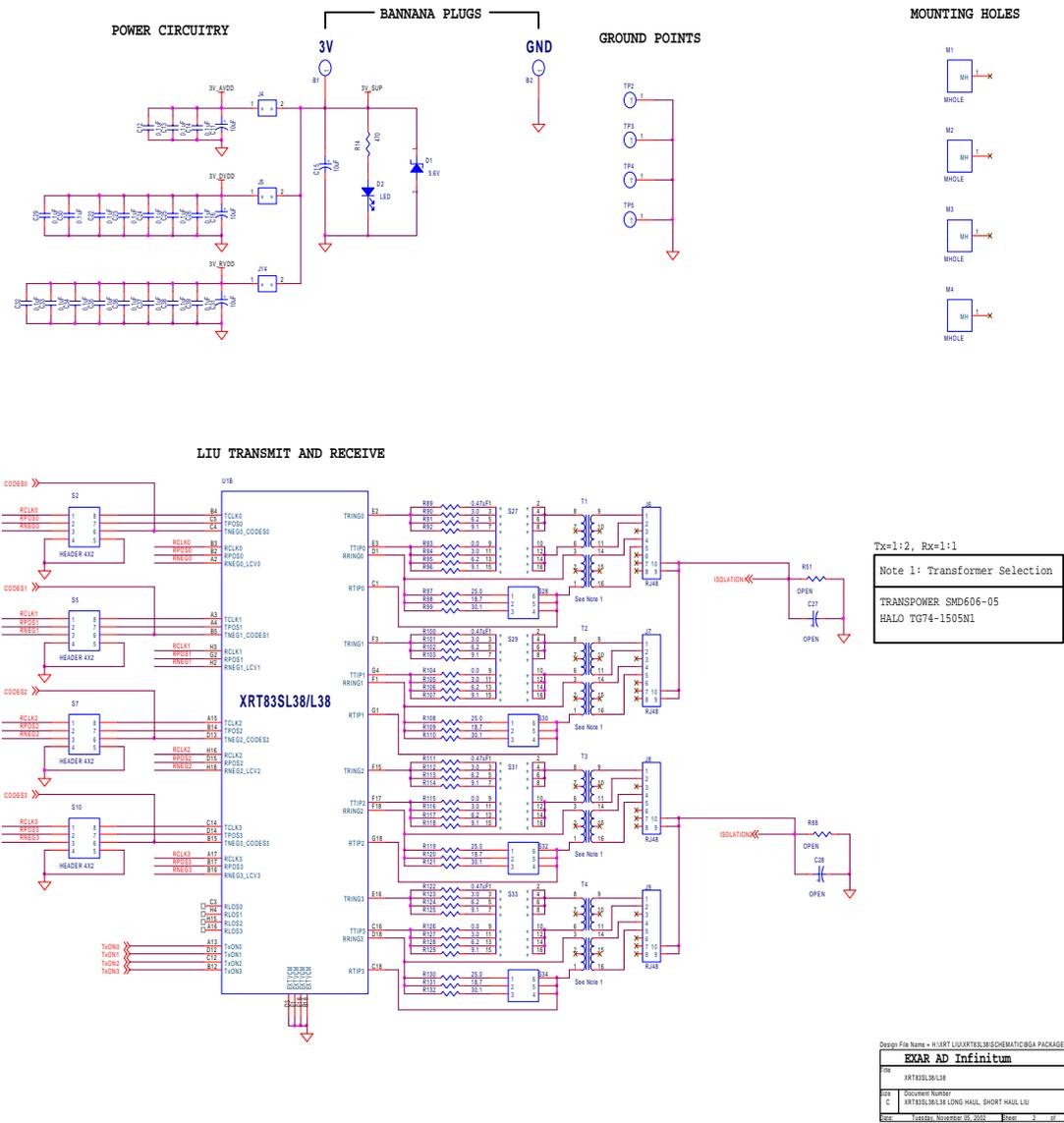
Figure 7 XRT83SL38/L38EVAL BGA Schematic Page 2
