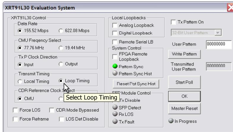
**Step 7.** Enable the Remote Serial Loopback by checking the on the “Remote Serial LB” box.
