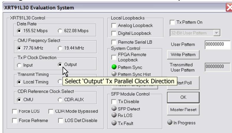
**Step 4.** Select **Local Timing** mode for the XRT91L30 transmit timing.
