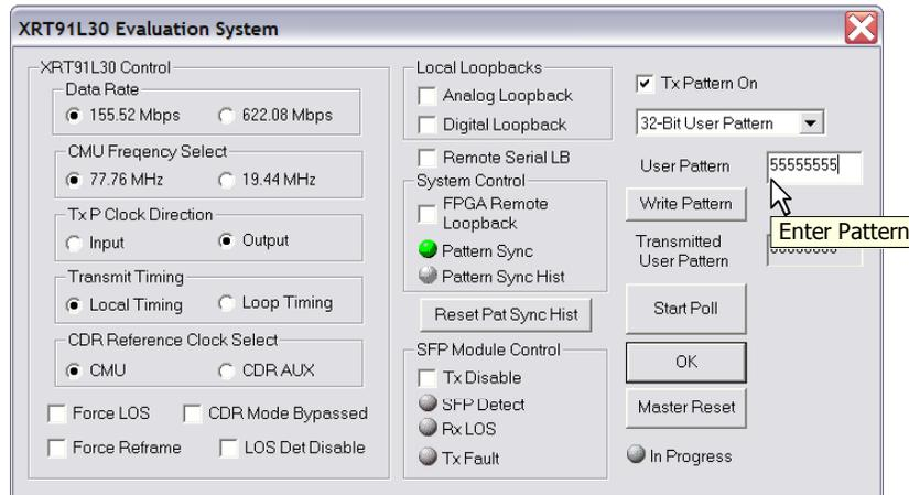
**Step 10.** Click on "Write Pattern" to load the user pattern into the FPGA buffer.
