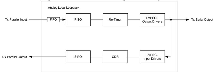
**Configuring for 2<sup>31</sup> – 1 PRBS pattern test using Analog Local Loopback Operation**
