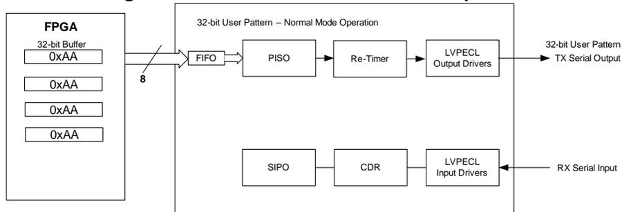
**Configuring the XRT91L30 for 32-bit User Pattern Transmission**
