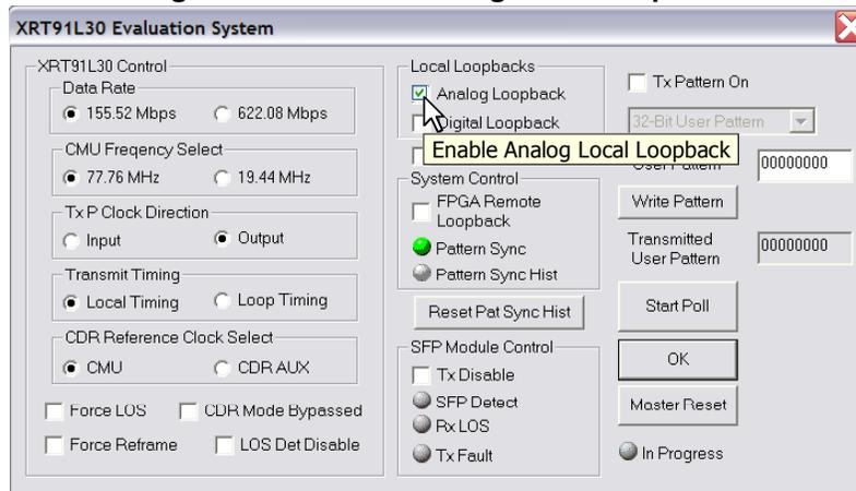
**Step 6.** To enable the transmission of pattern signal from the FPGA, check the “Tx Pattern On” box.
