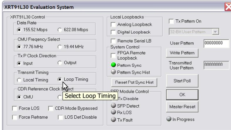
**Step 10.** Enable the FPGA Remote Loopback by checking the on the “FPGA Remote Loopback” box.
