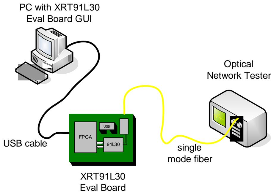
**Figure 7.9 Re-Verify Optical Signal Strength (Test Equipment)**
