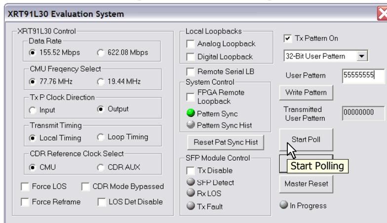
**Step 12.** Verify that the desired pattern is displayed on the “Transmitted User Pattern” window. This is the pattern currently transmitted by the XRT91L30.
