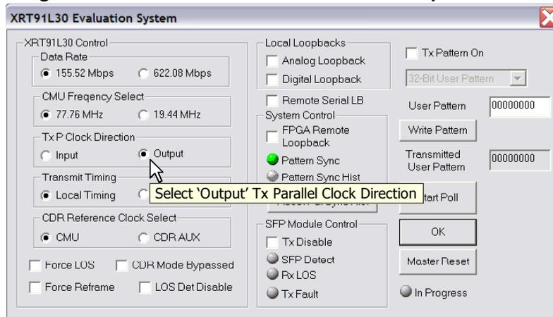
**Step 6.** Select **Local Timing** mode for the XRT91L30 transmit timing.
