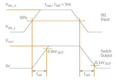
Figure 1. t<sub>ON</sub>, t<sub>OFF</sub>
