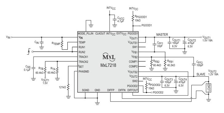
Figure 24: Example of Output Tracking Application Circuit
