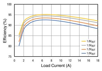
**Figure 4**: Efficiency: Single Phase, V<sub>IN</sub> = 5V, 450kHz
