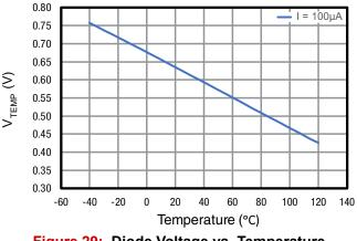
Figure 29: Diode Voltage vs. Temperature
