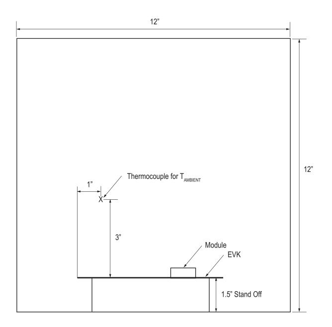
Figure 33: Current Derating Curves Measurement Setup
