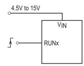
Figure 26: RUNx Pin Driven by a Logic Signal
