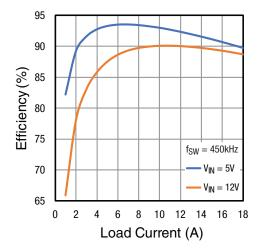
Figure 2: 1.2V<sub>OUT</sub> Efficiency vs I<sub>OUT</sub>
