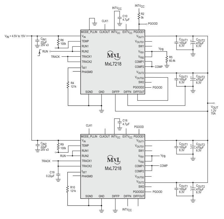
Figure 18: MxL7218 2-Module, 4-Phase, 1.2V, 70A Regulator
