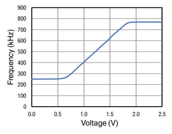
Figure 22: Operating Frequency vs. f<sub>SET</sub> Pin Voltage
