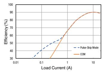
Figure 7: Efficiency: Pulse-Skipping Mode, V<sub>IN</sub> = 12V,  $V_{OUT}$  = 1.2V, 450kHz
