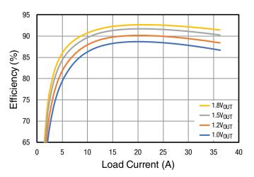
Figure 6: Efficiency: Dual Phase, V<sub>IN</sub> = 12V, 450kHz
