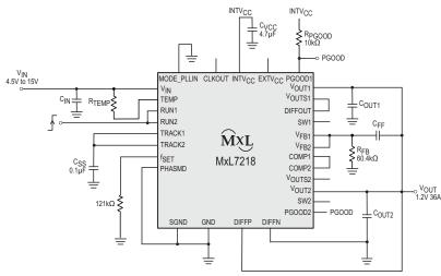
Figure 1: Typical Application: 36A, 1.2V Output DC/DC Power Module
