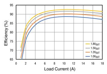
Figure 5: Efficiency: Single Phase, V<sub>IN</sub> = 12V, 450kHz
