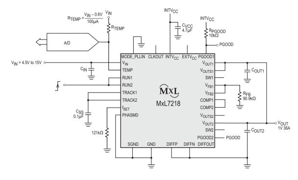
Figure 30: 2-Phase, 1V at 36A with Temperature Monitoring
