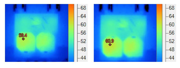
Figure 31: Thermal Image 12V to 1V, 36A with 200LFM<sup>(1)</sup>
