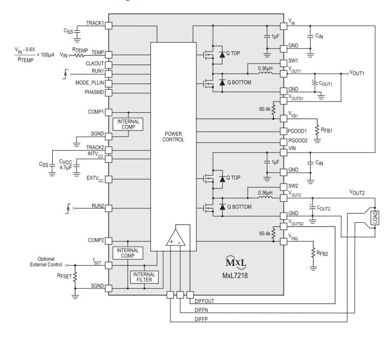
Figure 16: Functional Block Diagram
