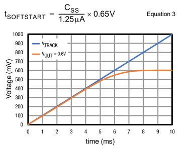
Figure 23: V<sub>OUT</sub> and V<sub>TRACK</sub> versus Time
