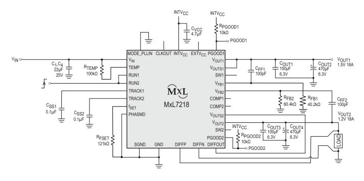
Figure 17: Typical 4.5V  $_{\rm IN}$  to 15V  $_{\rm IN},$  1.5V and 1.2V at 18A Outputs
