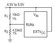
Figure 28: Self-Start for V<sub>IN</sub> Range of 4.5V to 5.5V
